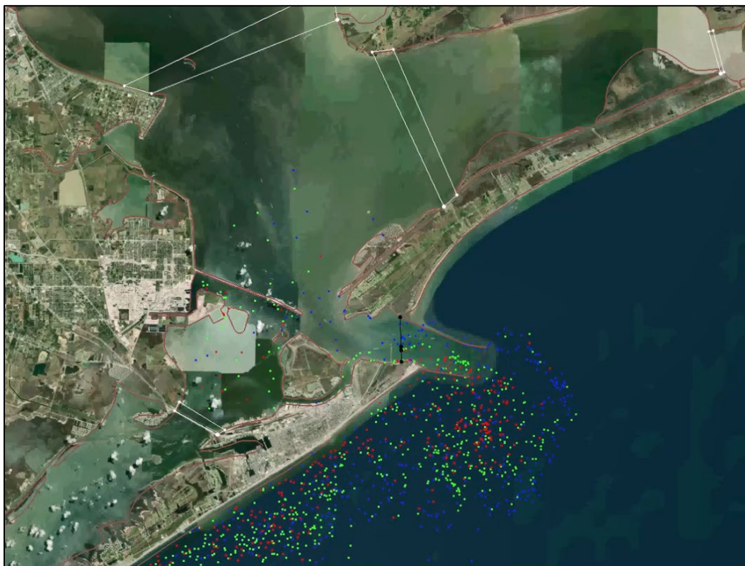
Figure 5-2. Particle position focused on transport along the shoreline .
