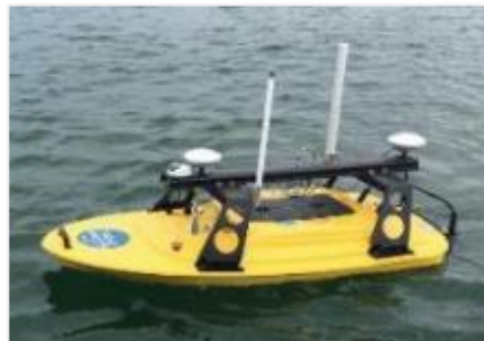
Remote Hydrographic Survey Vessel Z-Boat 1800 – dual channel, single beam SoNAR Utilized for shallow water surveys up to 1ft deep
