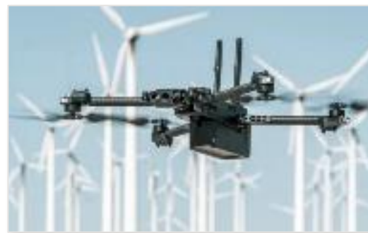
Skydio X2D – Color / Thermal Uses: Inspections, 4k Full Motion Video, photogrammetry
