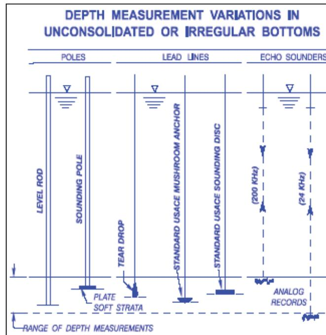
High-frequency echo sounders (200+ kHz) can reflect off the water/muddy water interface, and (given transmit and sensitivity settings are comparable) the lower frequency echo sounders can reflect off a density gradient (or density gradients) deeper in the fluid mud layer. This phenomenon is illustrated in Figure 17 that shows acoustic returns from a dual frequency echo sounder used by the Mobile District (41 and 200 kHz). The high
