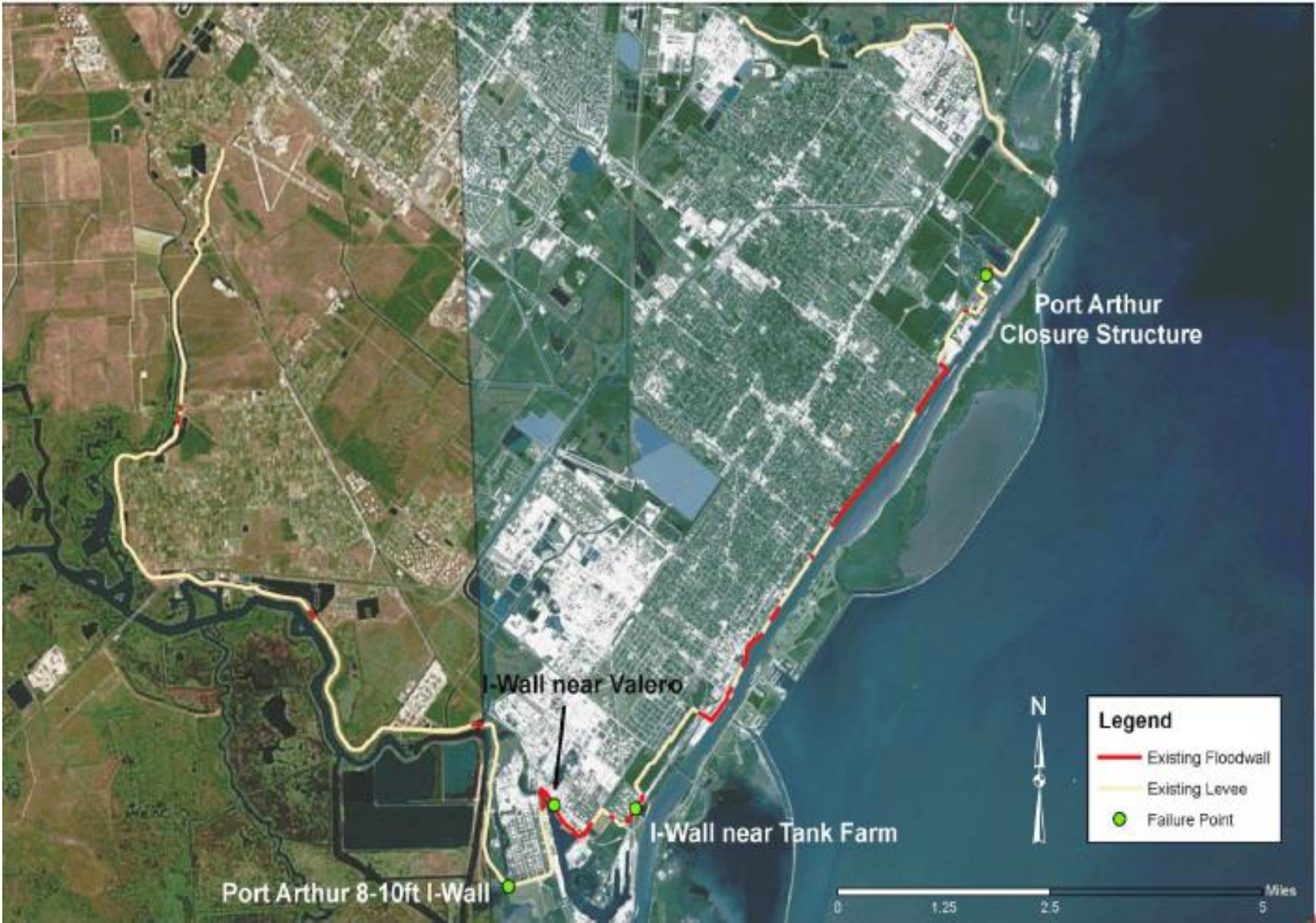
Figure 7-4. Port Arthur and Vicinity CSRM Failure Locations
