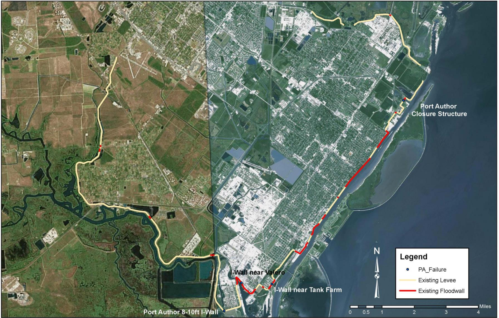
Figure 7-7. Port Arthur and Vicinity Failure Locations
