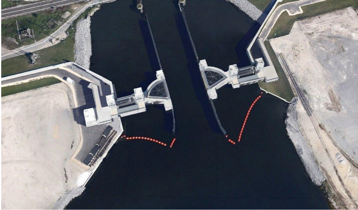
Figure 7-1. Conceptual Plan View of Adams and Cow Bayou Structures
