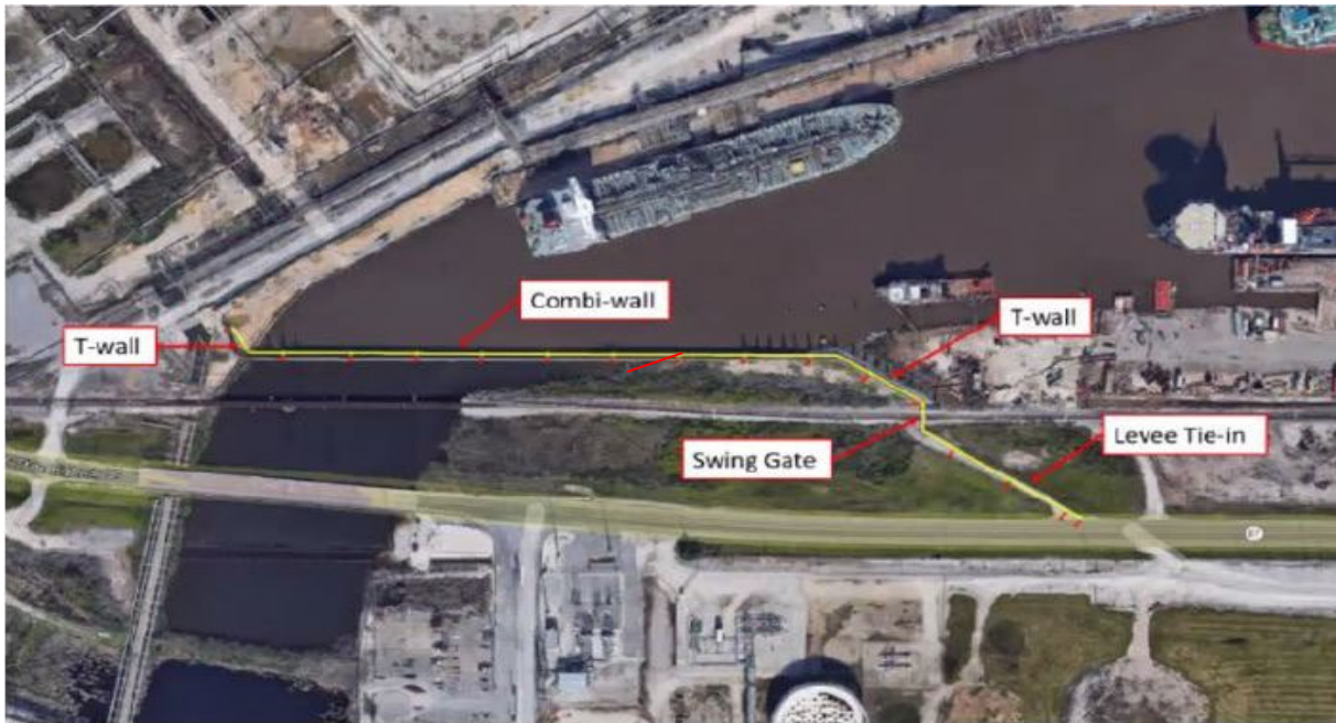
Figure 2: Existing Levee-Floodwall System
