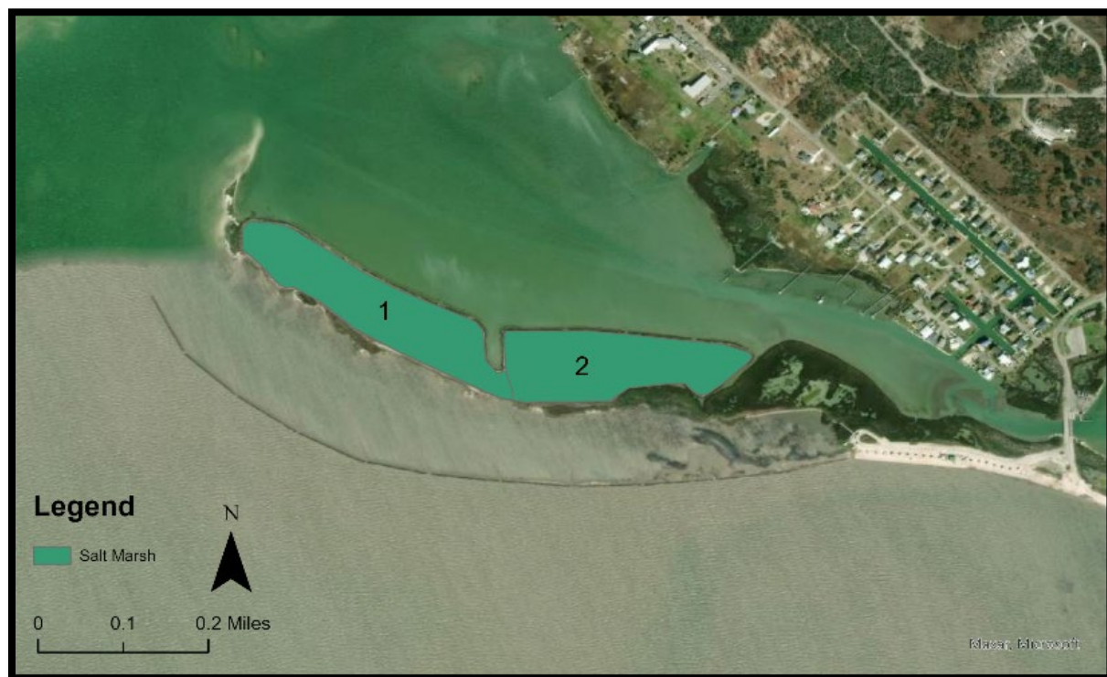
Figure 8: Alternative 3A builds 23 acres of saline marsh targeting 0.6 to 0.8 ft final elevation.
