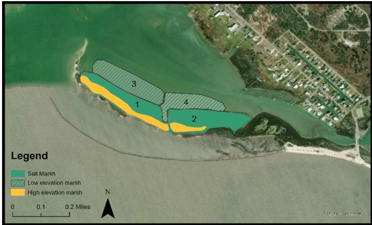
Figure 10: Alternative 3C constructs a 32.5 acres of low elevation marsh (0.6 to 0.8 ft NAVD88) and 6.5 acres of high elevation marsh (1.5 to 2.0 ft NAVD88)
