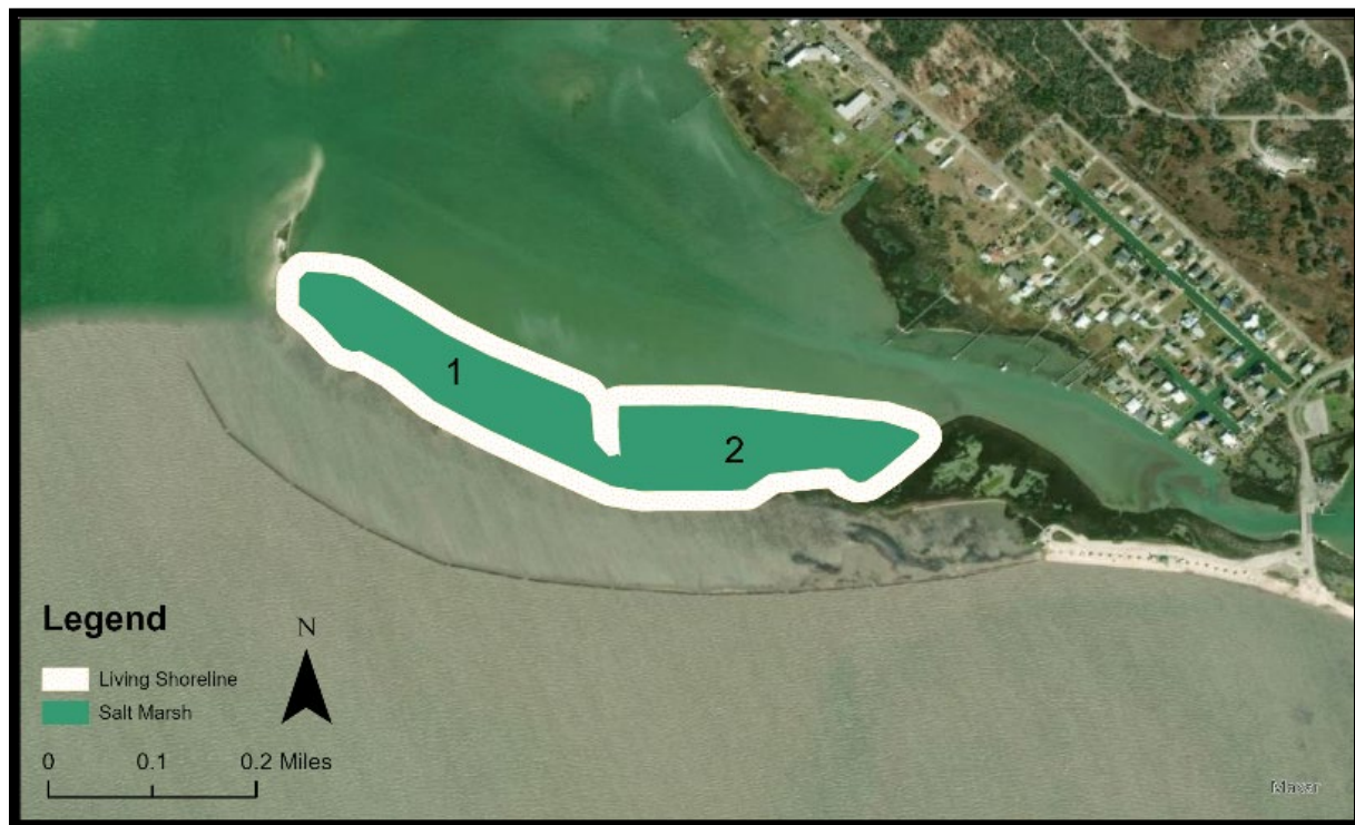
Figure 9: Alternative 3B builds 23 acres of saline marsh (final elevation = 0.6 to 0.8 ft NAVD88) with a living shoreline
