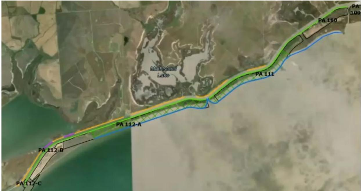
Increment 1 – The Bayside Breakwater (blue line in above figure) will be constructed about 3 feet above the MSL elevation, and sediment placement and marsh planting will fill the area inside (green hatching in above figure).
