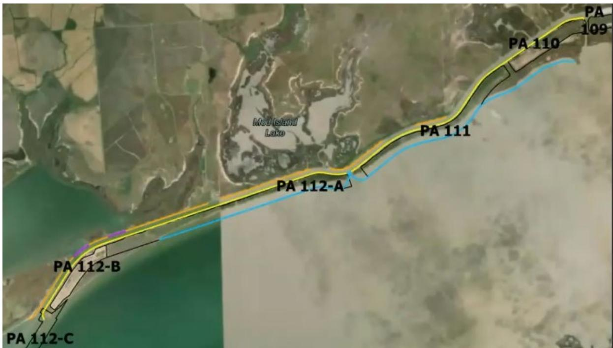
Increment 1 – The Bayside Breakwater (light blue line in above figure) will be constructed about 5 feet above the MSL elevation.
