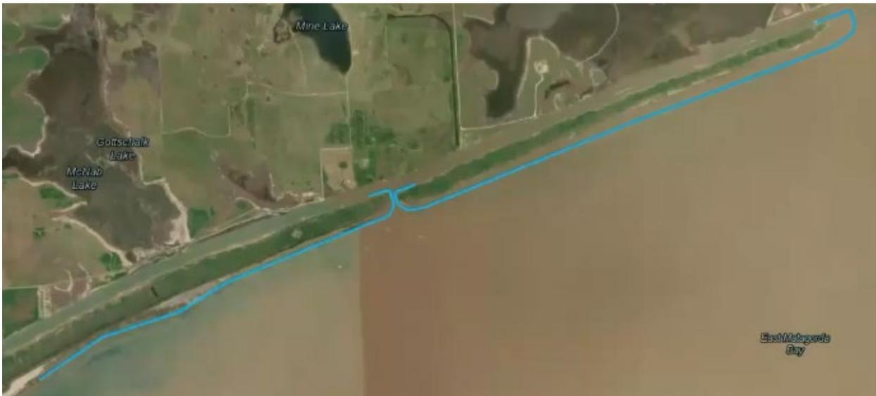
Increment 1 – Bayside Breakwater (light blue line in above figure) will be constructed about 5 feet above the MSL elevation. The Channel Bayside and Landside Breakwaters were screened earlier in the study due to the shoaling rate not being significant enough from the H&H analyses. This can be further evaluated later to confirm whether there is a need for Channel Landside Breakwaters for PA 105.
