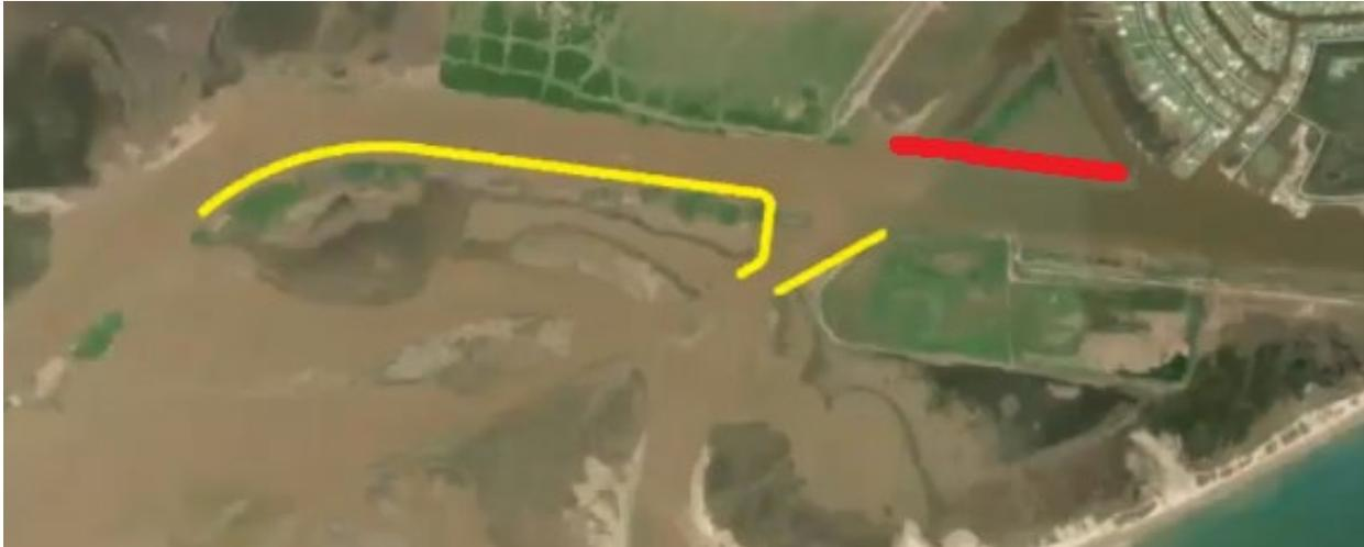
Increment 1 – Channel Bayside Breakwater (yellow lines in above figure) which will be constructed about 7 feet above the mean sea-level (MSL) elevation. Channel Landside Breakwaters are excluded from this zone because they are included as part of the Coastal Texas Protection and Restoration Study.
