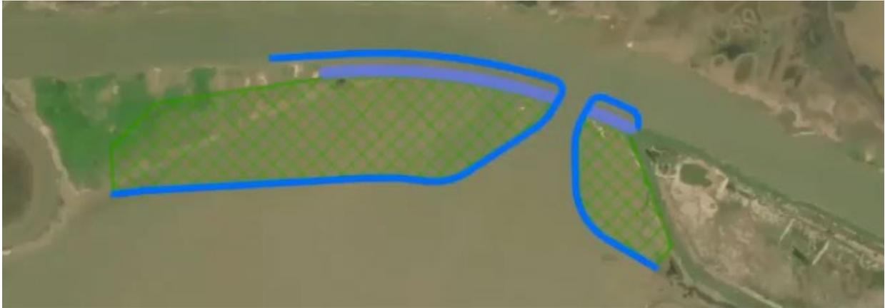
Increment 1 – The Channel Bayside Breakwater and Bayside Breakwater (blue line in above figure) will both be constructed to be about 3 feet above the MSL elevation, and sediment placement and marsh planting will fill the inside area (green hatching in above figure). Also, there will be an earthen berm just on the inside of the Channel Bayside Breakwater (purple line in above figure).
