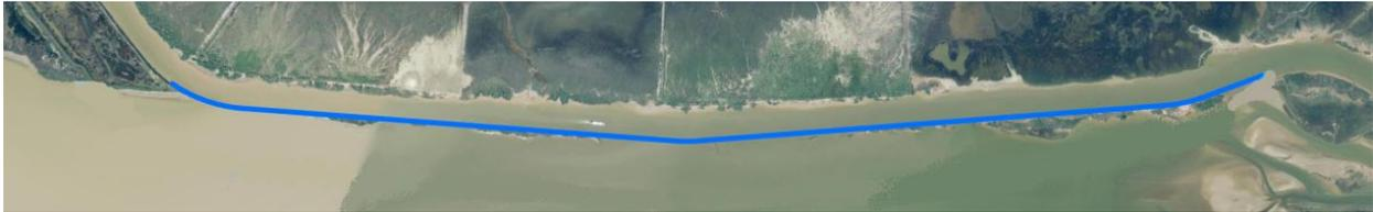
Increment 1 – Channel Bayside Breakwater (blue line in above figure) will be constructed about 7 feet above the MSL elevation. There are no further increments for this alternative because the barrier islands will be completely eroded away and/or submerged by 2030 which is the proposed start date of construction. Also, Channel Landside Breakwaters are excluded from this zone because they are included as part of the Coastal Texas Protection and Restoration Study.
