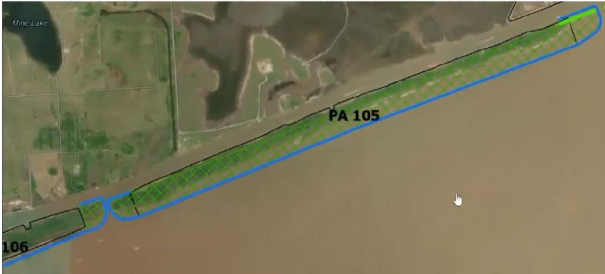
Increment 1 – The Bayside Breakwater (blue line in above figure) will be constructed in the same location as alternative 3 but at a height of about 3 feet above the MSL elevation, and sediment placement and marsh planting will fill the area in PA 105 and on the edge of PA 106 (green hatching in above figure). Also, there will be a small earthen berm on the inside of the curved edge of the Bayside Breakwater wrapping around to the channel side (light green line in above figure).
