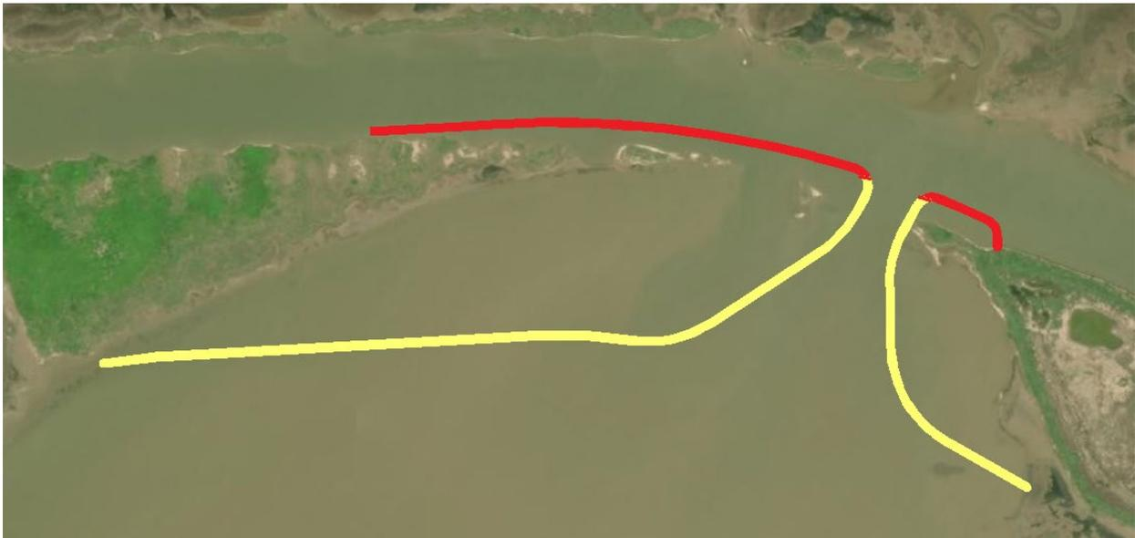
Increment 1 – Bayside Breakwater (yellow line in above figure) will be constructed about 5 feet above the MSL elevation, and Channel Bayside Breakwater (red line in above figure) will be constructed about 3 feet above MSL elevation. Channel Landside Breakwaters are excluded from this zone because they are included as part of the Coastal Texas Protection and Restoration Study.
