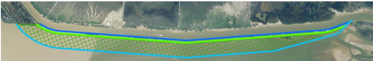
Increment 1 – The Channel Bayside Breakwater (blue line in above figure) and the Bayside Breakwater (light blue line in above figure) will both be constructed to be about 3 feet above the MSL elevation, and sediment placement and marsh planting (green hatching) to fill the area between the two breakwaters which is about 405 acres. Also, there will be an earthen berm (light green line in above figure) just on the inside of the Channel Bayside Breakwater.
