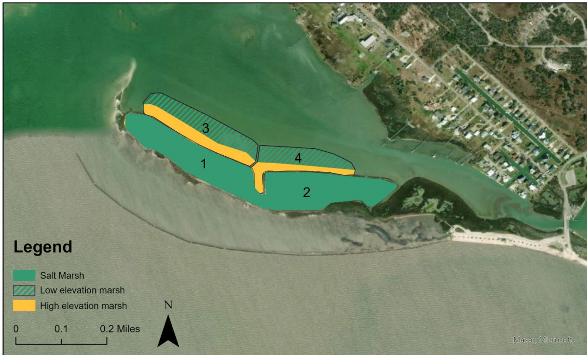
Figure 2. Alternative 3D, the proposed marsh restoration for Goose Island State Park. Salt marsh and low elevation marsh will target +0.6 to +0.8-feet NAVD88 (+1.5 to +1.7-feet MLLW) final elevation and high elevation marsh will target +1.5 to +2.0-feet NAVD88 (+2.4 to +2.9-feet MLLW)
