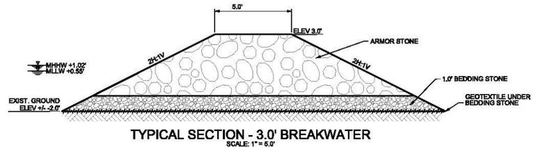
TYPICAL SECTION - 3.0' BREAKWATER
