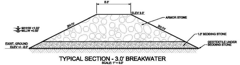
TYPICAL SECTION - 3.0' BREAKWATER
