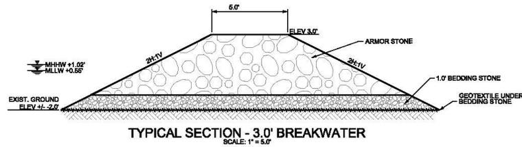
TYPICAL SECTION - 3.0' BREAKWATER
