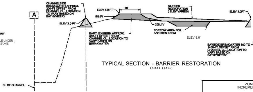
TYPICAL SECTION - BARRIER RESTORATION (NOT TO SCALE)
