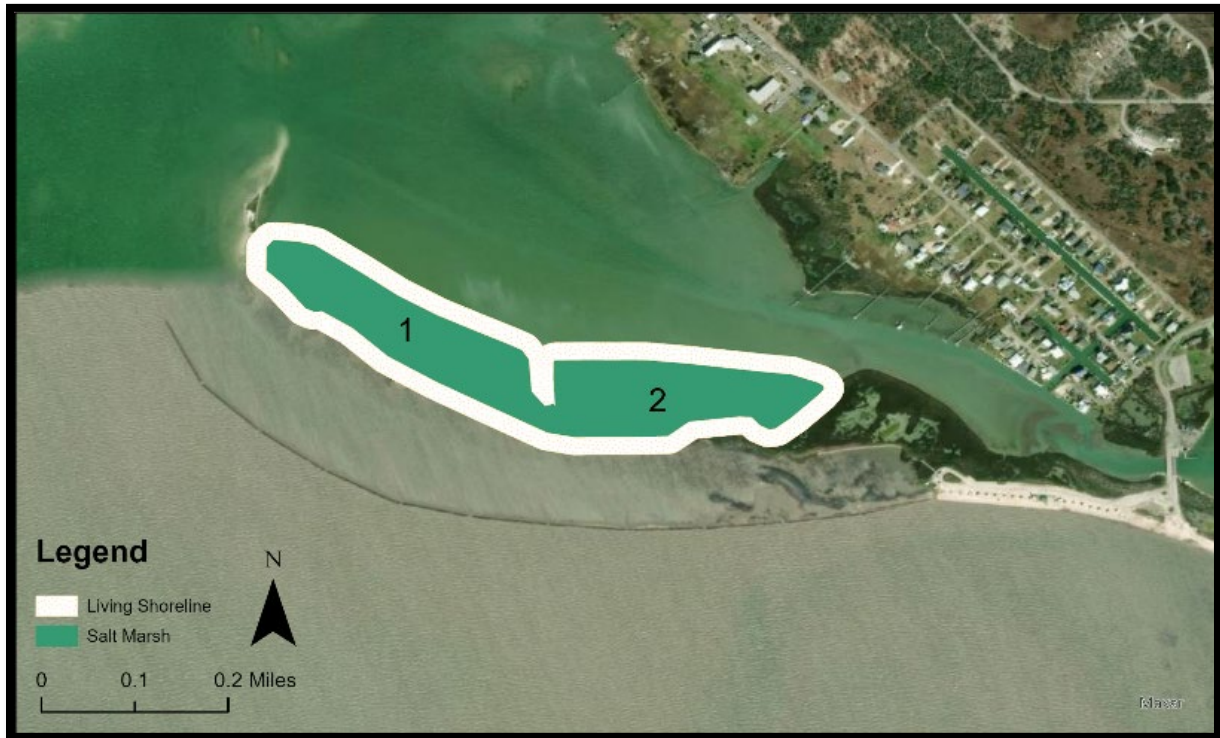
Figure 11: Alternative 3B builds 23 acres of saline marsh (final elevation = 0.6 to 0.8 ft NAVD88) with a living shoreline
