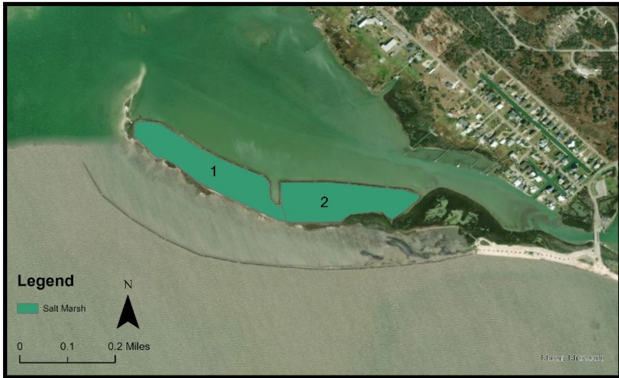
Figure 10: Alternative 3A builds 23 acres of saline marsh targeting 0.6 to 0.8 ft final elevation.
