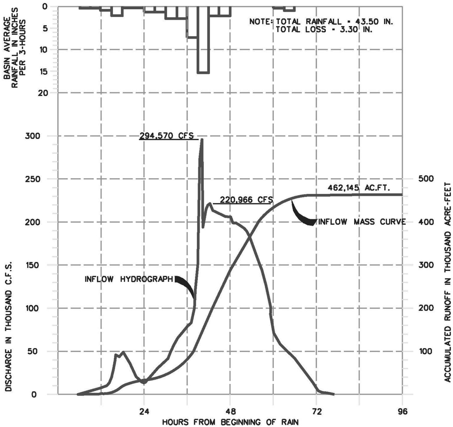
1977 Spillway Design Flood - Addicks Reservoir
