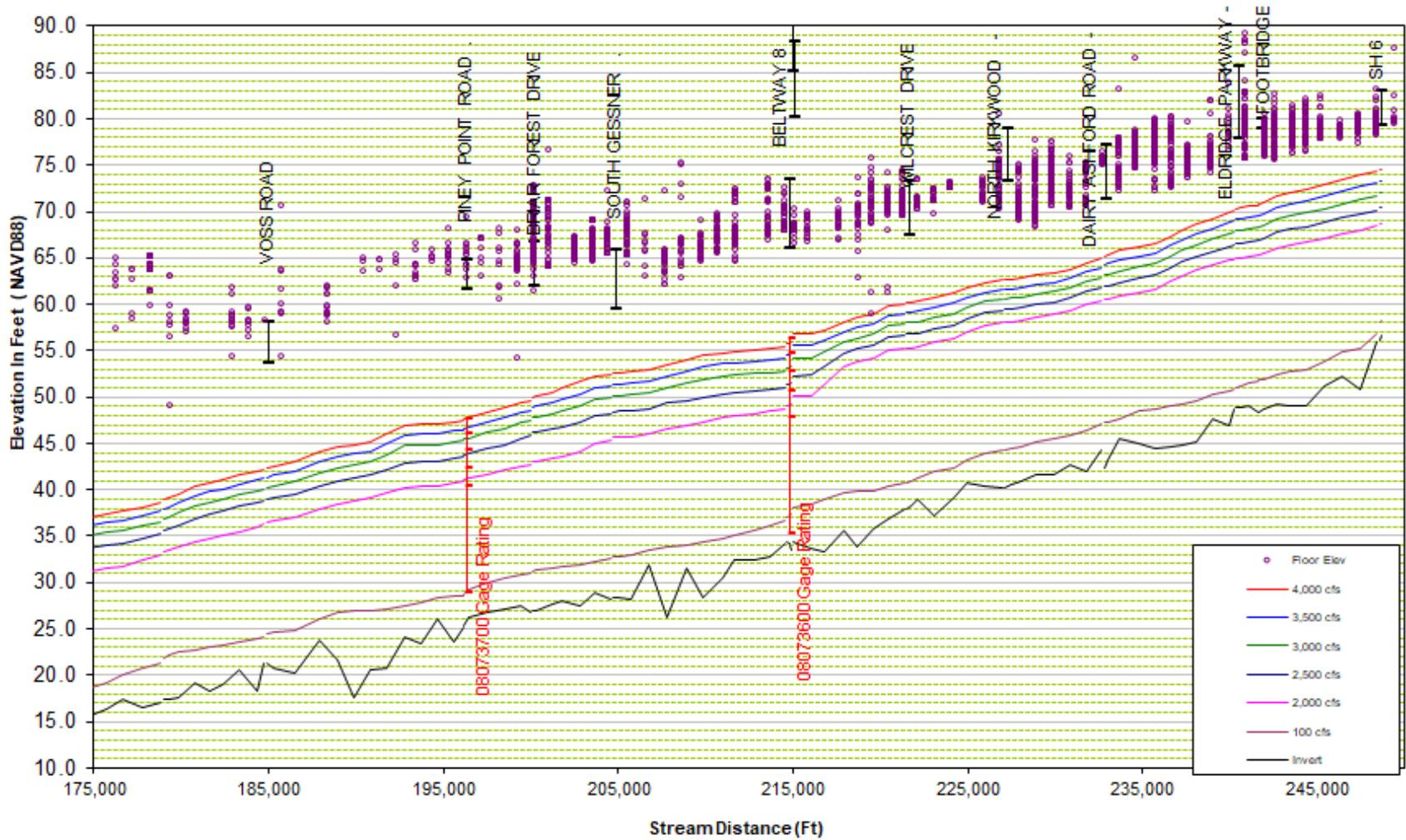
**Water Surface Profiles and Floor Elevations
