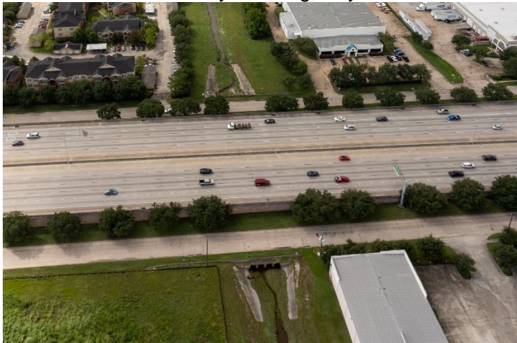
Figure 7. Culvert transition from roadside ditch under Beltway 8 in Houston, TX (Source: Molly Ross)
