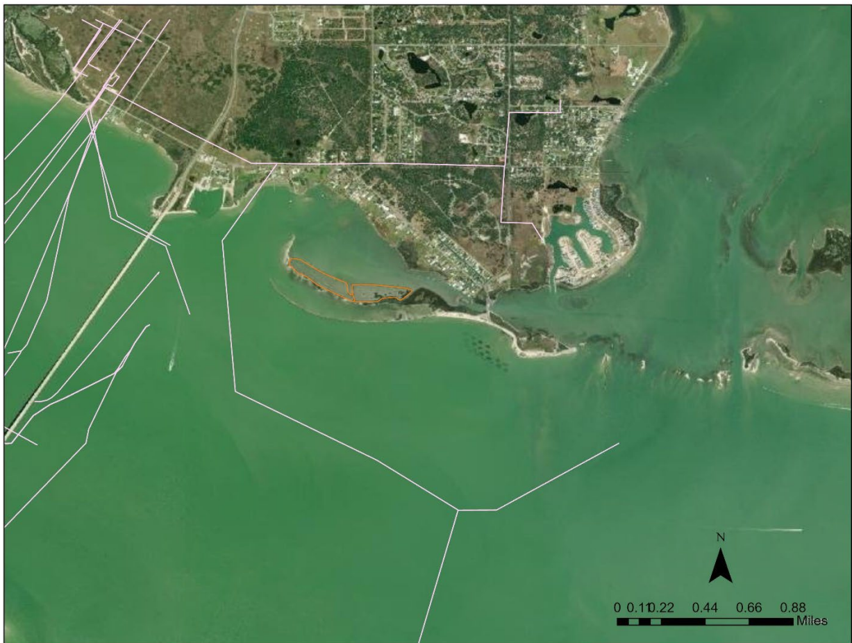
Figure 7- Pipelines in the Project Vicinity
