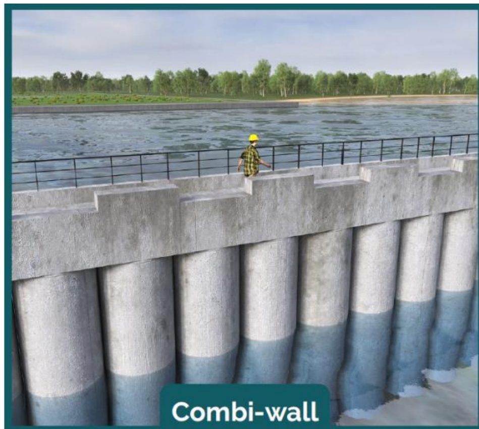
Figure 6-5: Combi-wall (Conceptual Rendition)
