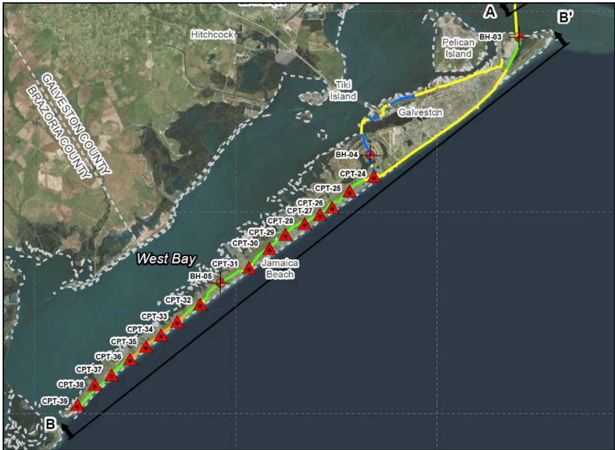
Figure 3-10: Boring Plan on Galveston Island (Sea Wall to San Luis Pass) (Source: GCCPRD, 2017)
