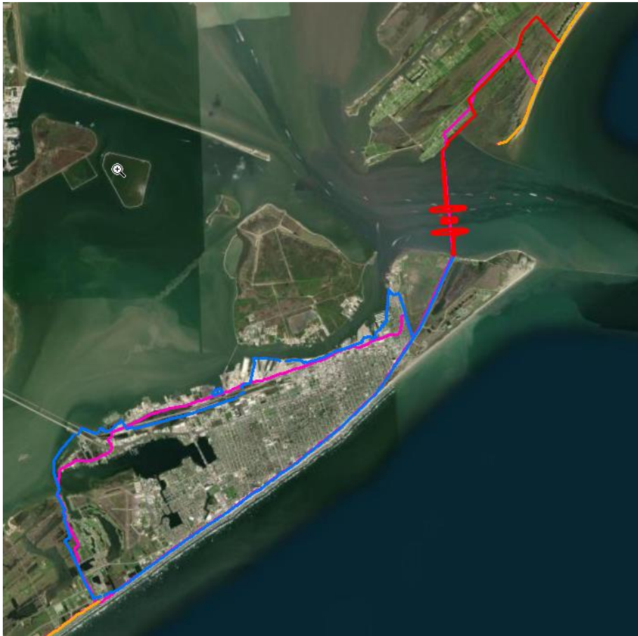
Figure 2-41: Difference in Barrier Alignment between TSP and Storm Surge Model (Orange is Beach & Dune System, Red is Bolivar Road Surge Barrier System, and Blue is Galveston Ring Barrier System)
