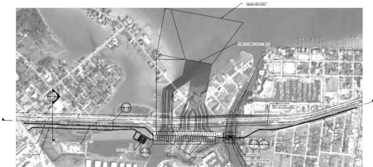
Figure 2-53: Clear Lake Gate Closure System with Pump Station Footprint (Annex 7 has details)
