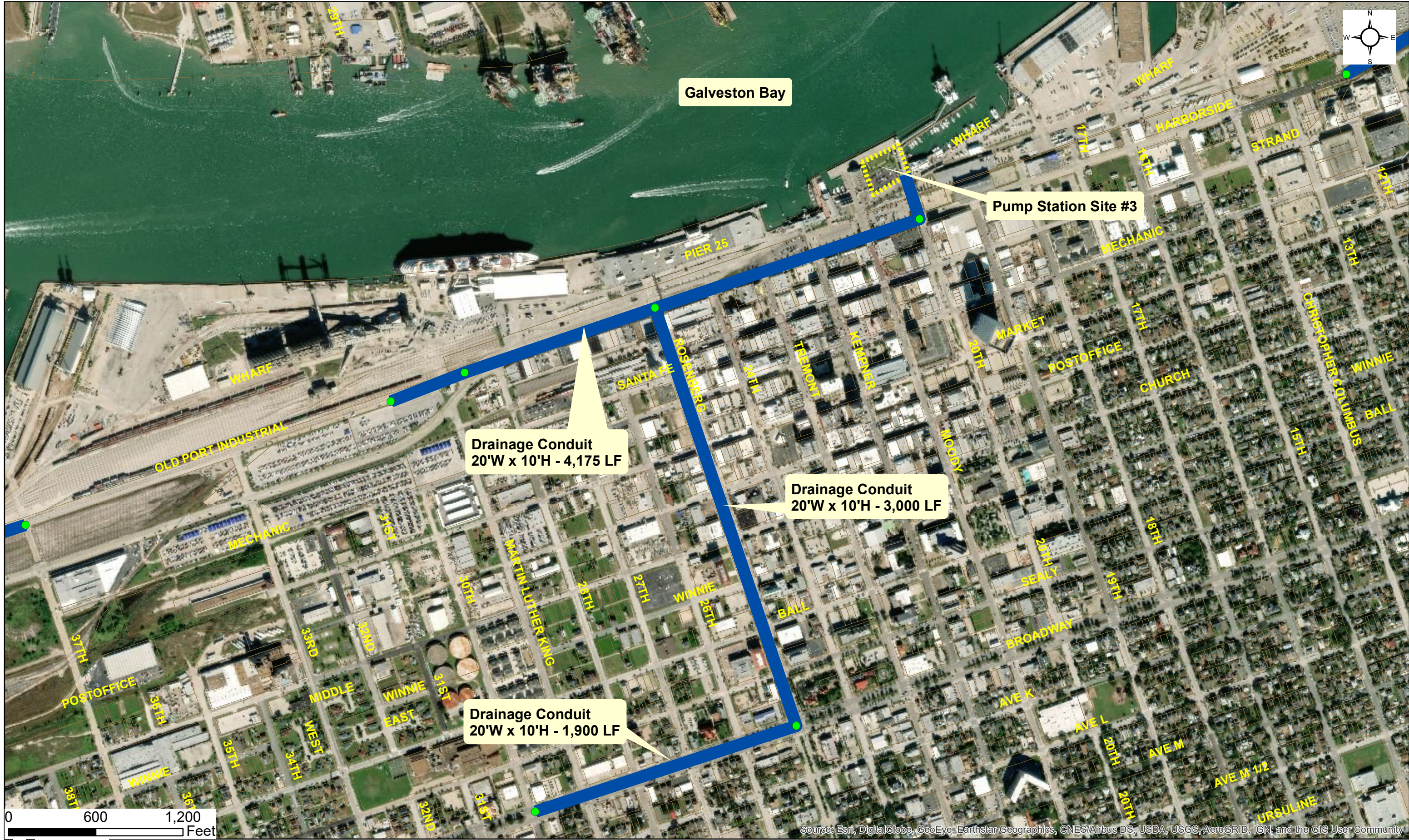
Proposed Stormwater Conduit and Potential Pump Station Site #3 City of Galveston, Texas.
