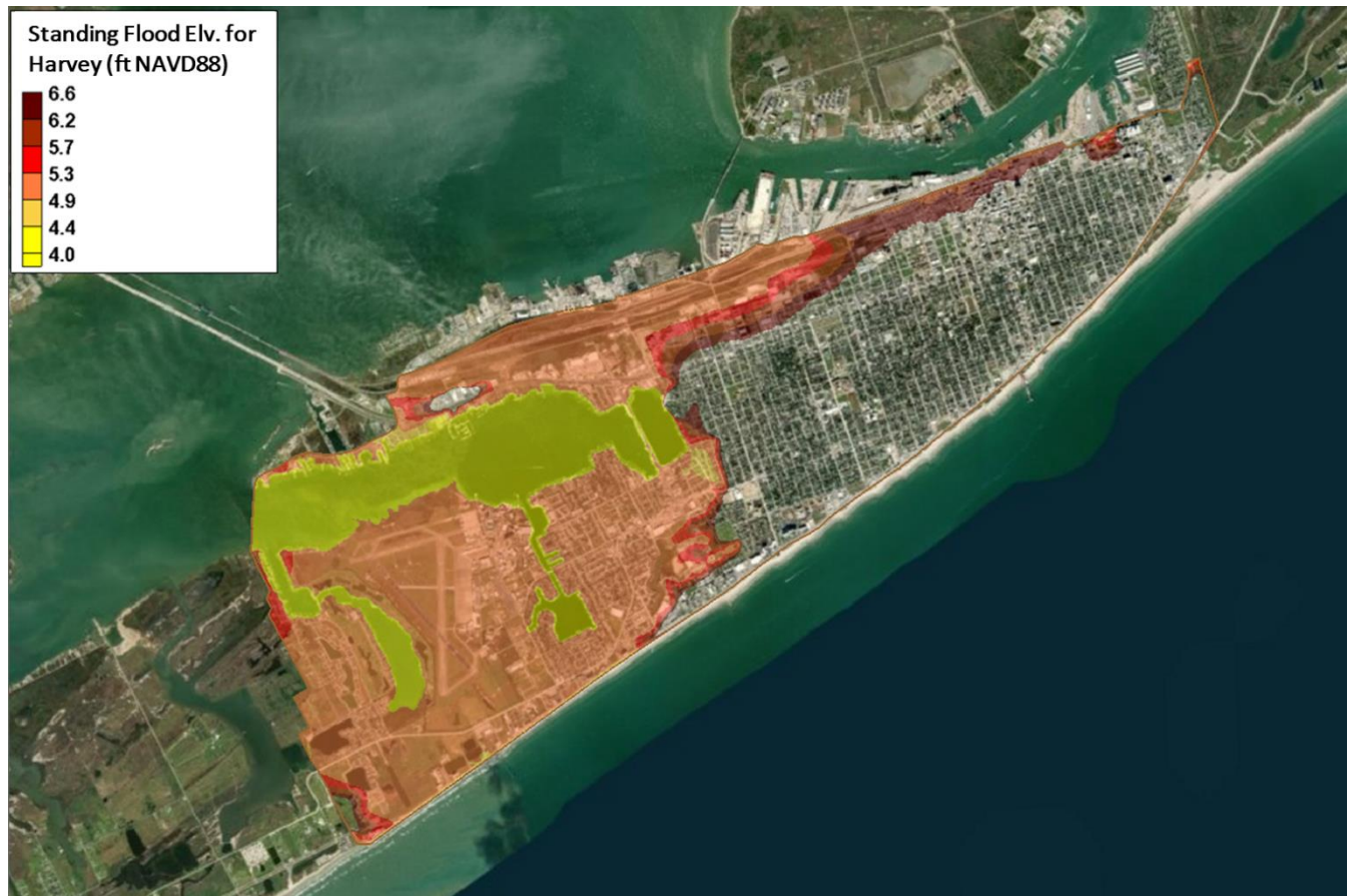
Figure 56. Flood coverage at elevation 6.6 ft NAVD88 for the Case 1 simulation using the Harvey rainfall.
