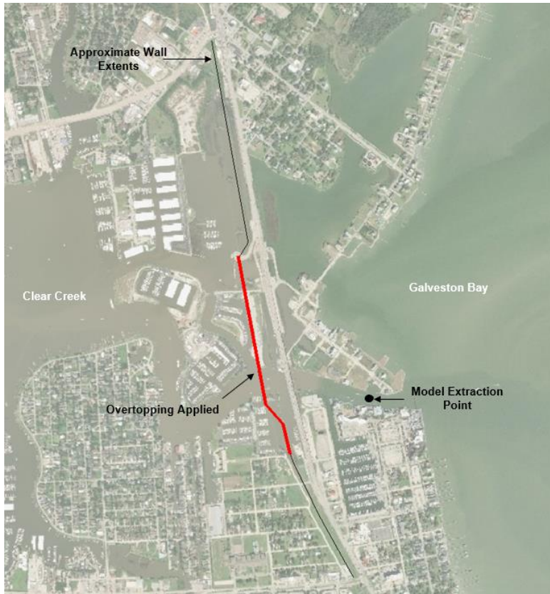
Figure 20. Model extraction point and representative wall length where overtopping was applied (red). Approximate wall extents also shown (black).
