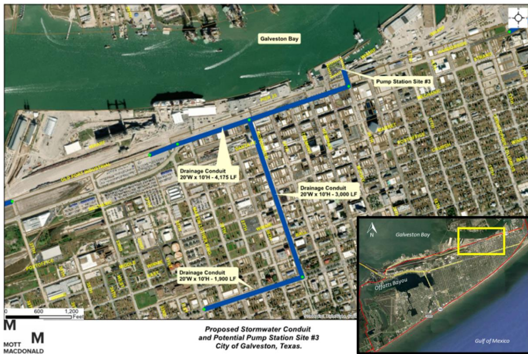
Figure 9. Original proposed stormwater conduit into Pump Site 3.
