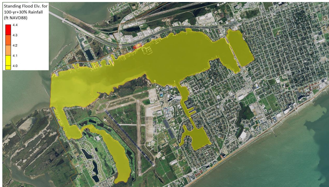
Figure 54. Standing flood coverage at elevation 4.4 ft NAVD88 from the 100-yr+30% rainfall with the 25-yr+30% facilities.
