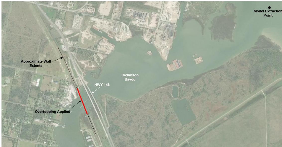
Figure 38. Model extraction point and representative wall length where overtopping was applied (red). Approximate wall extents also shown (black).
