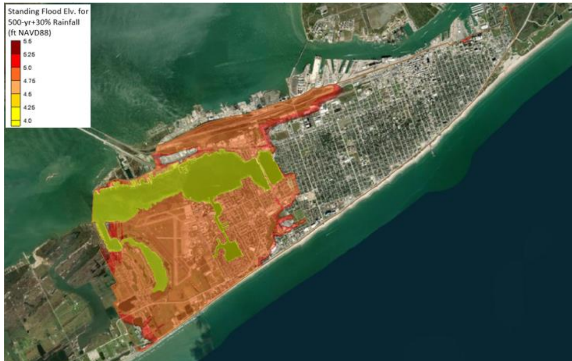
Figure 55. Standing flood coverage at elevation 5.5 ft NAVD88 from the 500-yr+30% rainfall with the 25-yr+30% facilities.
