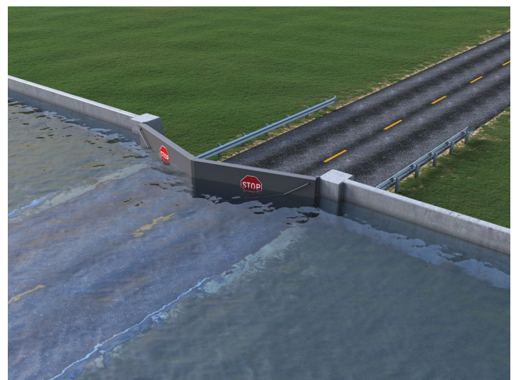
Conceptual rendering of highway flood gate proposed as part of the Galveston Ring Barrier System
