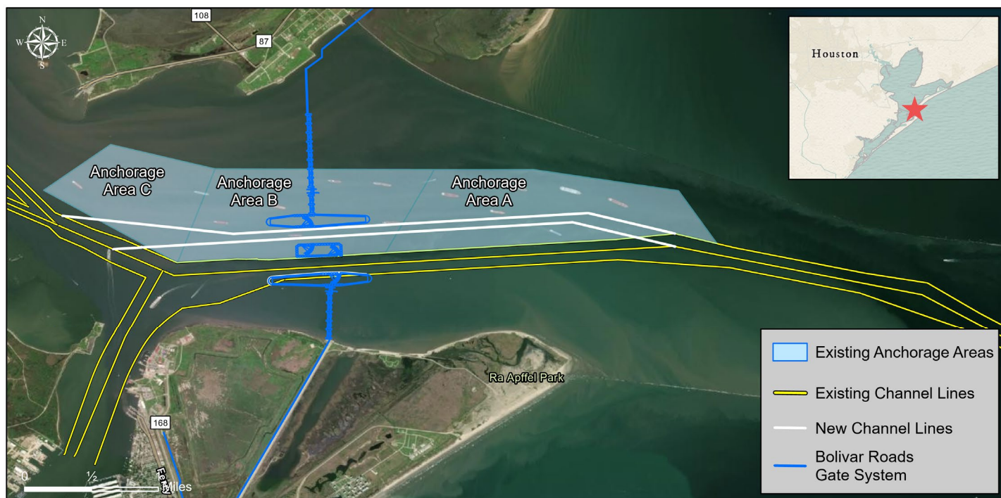
Figure 3.24: Bolivar Roads channel configuration
