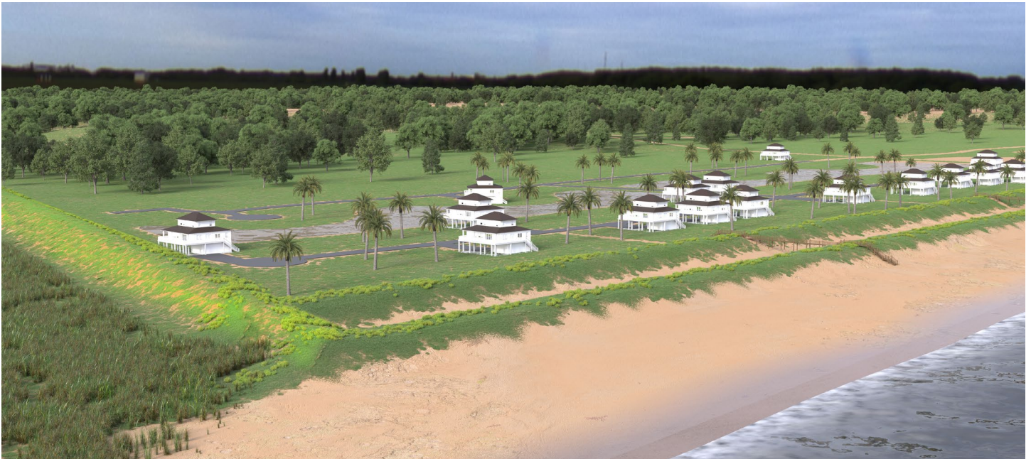
Conceptual rendering depicting the Bolivar dune system connected to the proposed levee system
