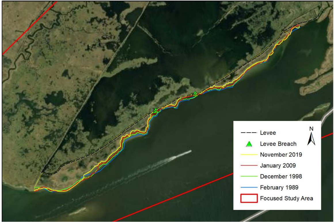
Figure 20. Shoreline Change from 1989 to 2019 at Hickory Cove based on Aerial Imagery
