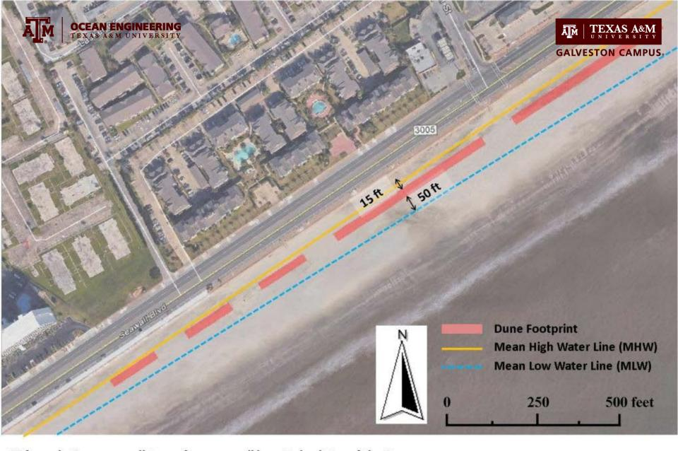
15 ft mark: An average distance from seawall base to back toe of the Dune 50 ft mark: An average distance from front toe of the Dune to MLW
