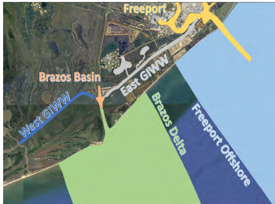
Figure 3-4 - BRFG Sediment Deposition Areas
