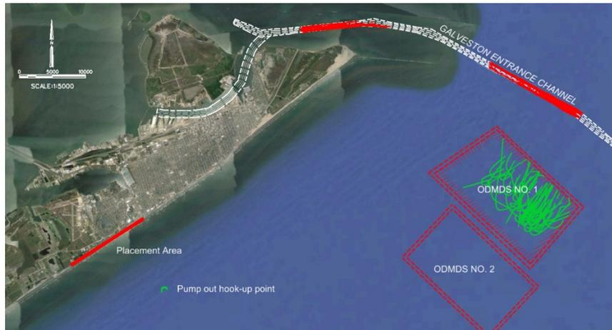
Fig. 4. Galveston Entrance channel dredging 2015 and placement locations. DQM dredging location data is shown in red in the channel, and green shows placement and pump out locations.
