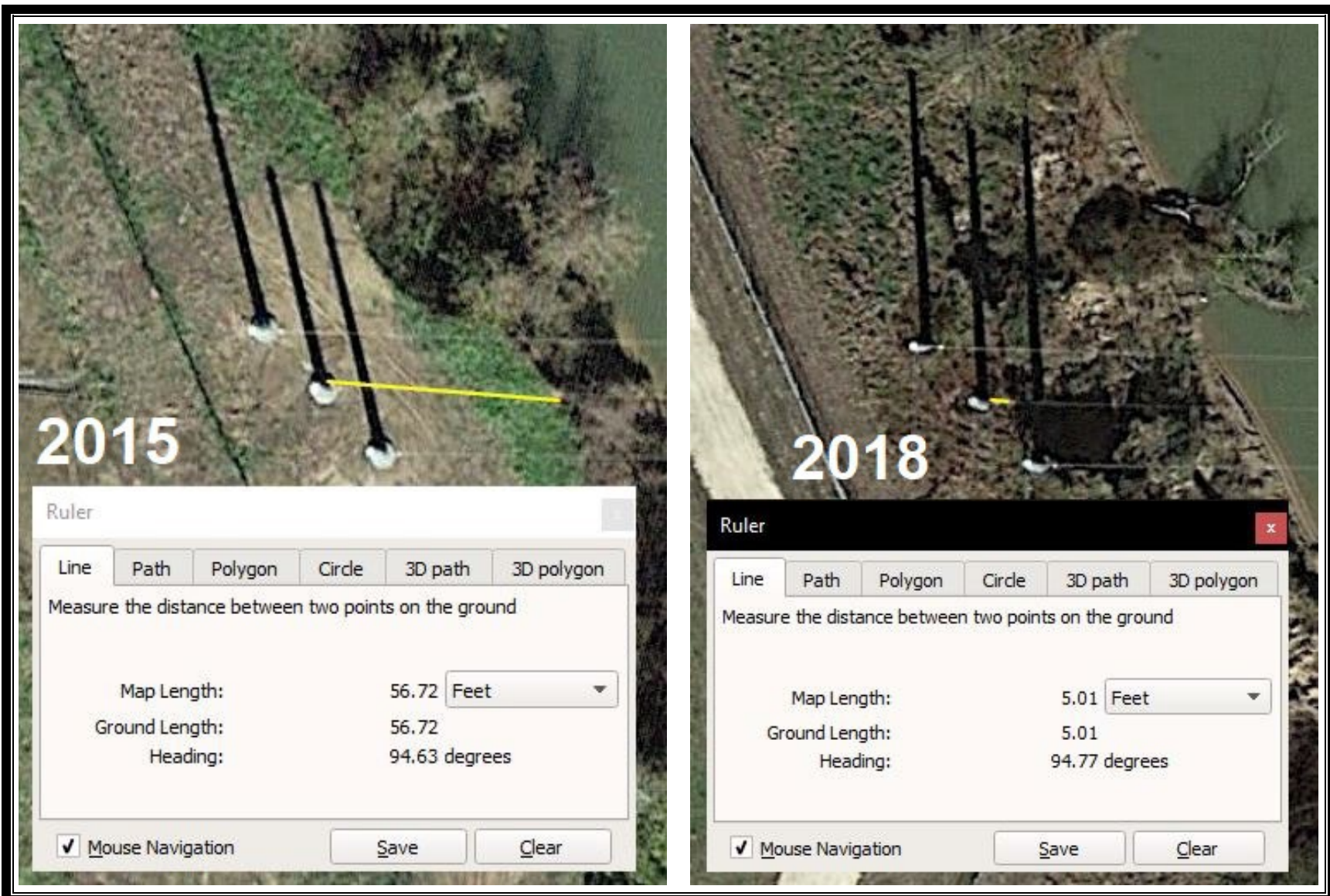
Figure 5 - Bank Erosion Measurement Site Four – 51 ft eroded in three years
