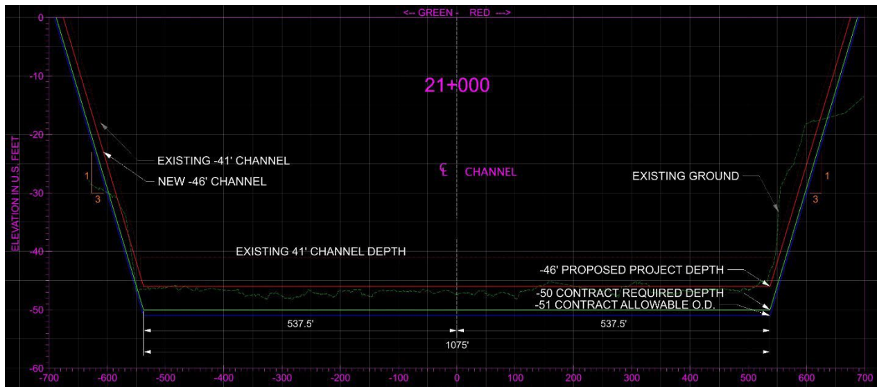
1 Cross-Section Template Sample of Modified Plan
