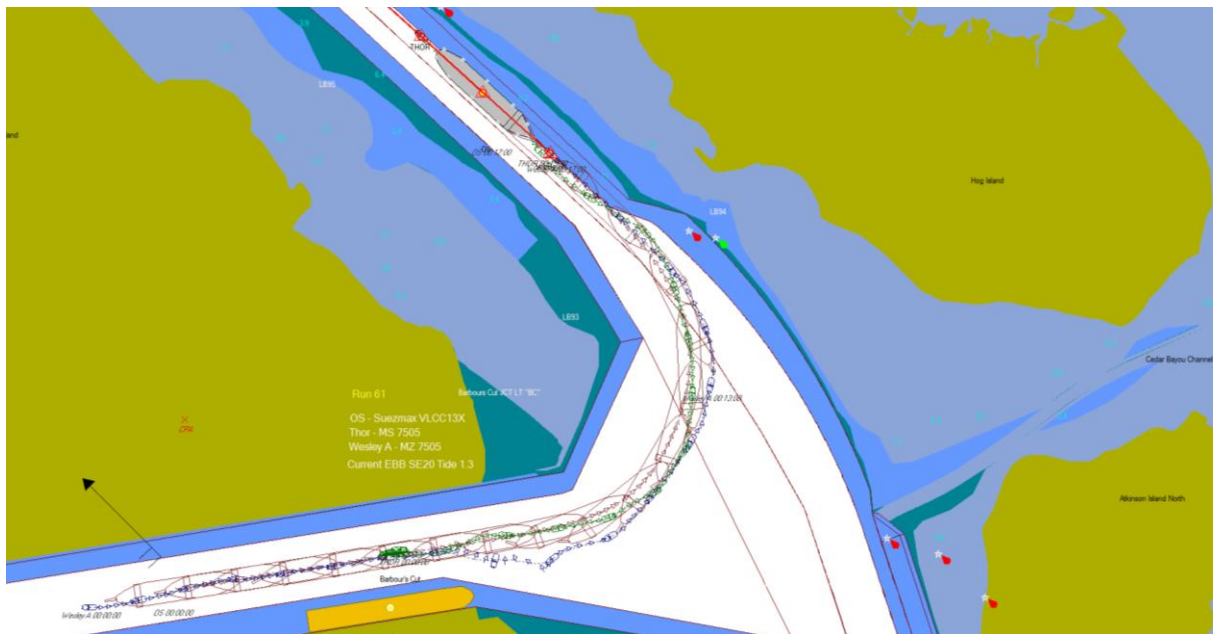
Figure 11. Suezmax Exiting the Barbours Cut Container Terminal Channel and Turning Up-channel Using the Widening Flare and East Houston Ship Channel Widener at Markers 83-84
