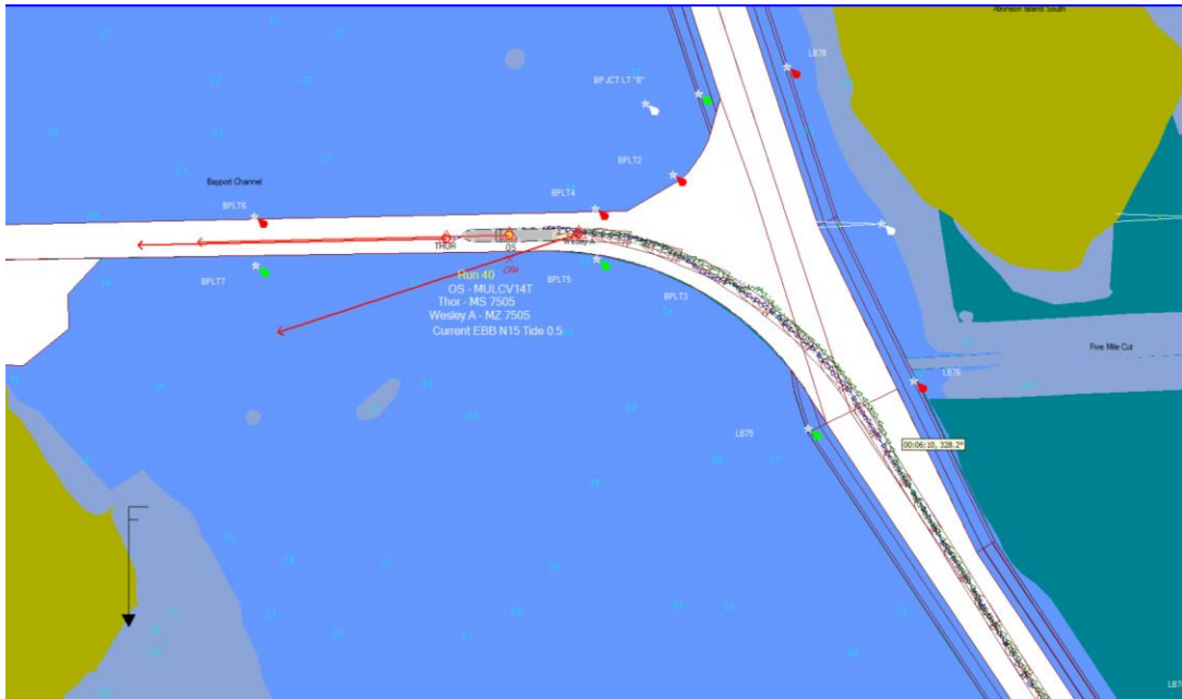
Figure 6. Design Containership Inbound to Bayport Container Terminal at Channel Intersection with HSC
