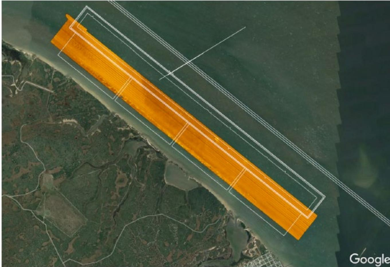
Figure 2. Basemap of MB2 survey area (NP2/OP2-5) with side scan sonar mosaic showing portions surveyed to date.
