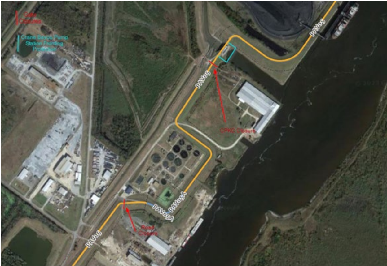
Figure 7: Pump Station Protection and Road Closure
