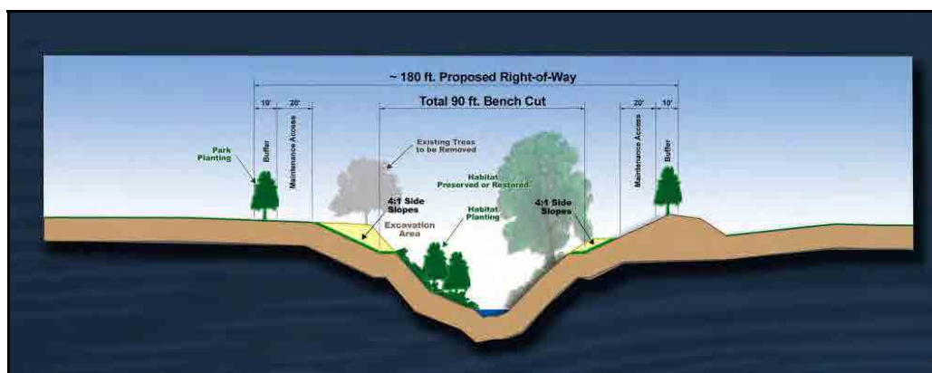
Figure 39. Illustration depicting on-the-ground designs for the Clear Creek Mainstem-Downstream Conveyance measure [C5(d)].
