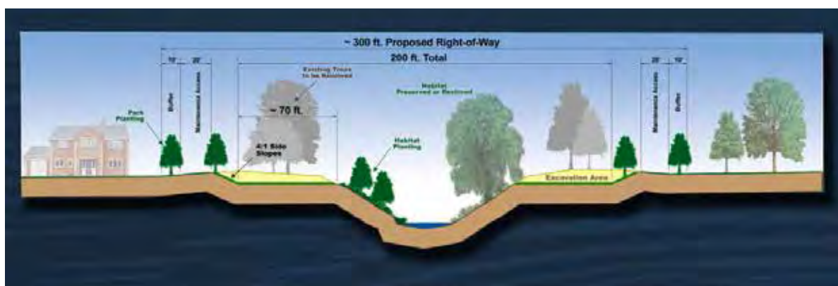
Figure 2.3-6. Super C(d) Conveyance Measure Cross Section
