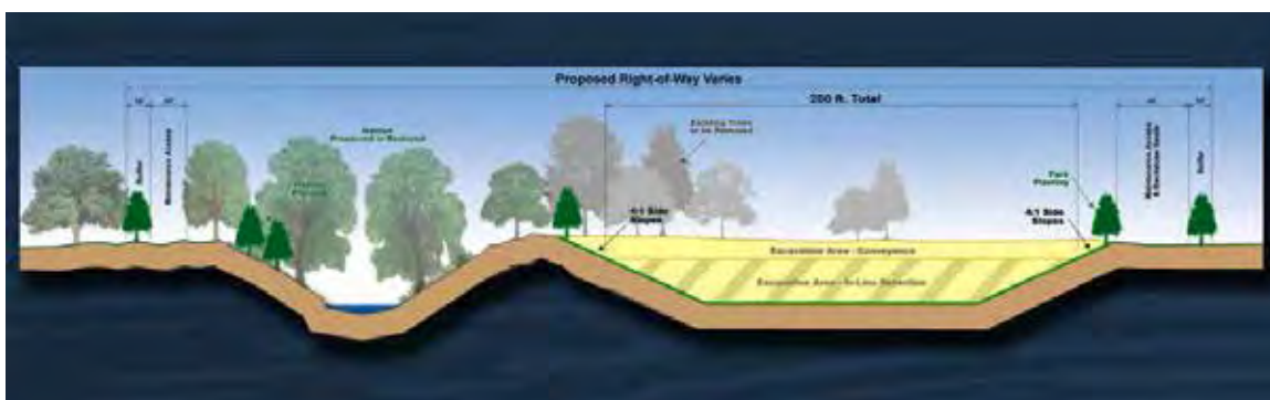
Figure 2.3-8. Clear Creek In-Line Detention Measure Cross Section
