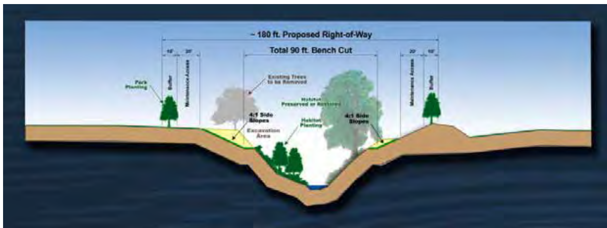
Figure 2.3-7. C5(d) Conveyance Measure Cross Section
