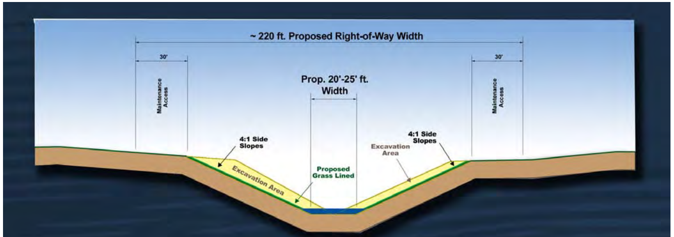
Figure 26 Turkey Creek Conveyance Measure Cross-Section
