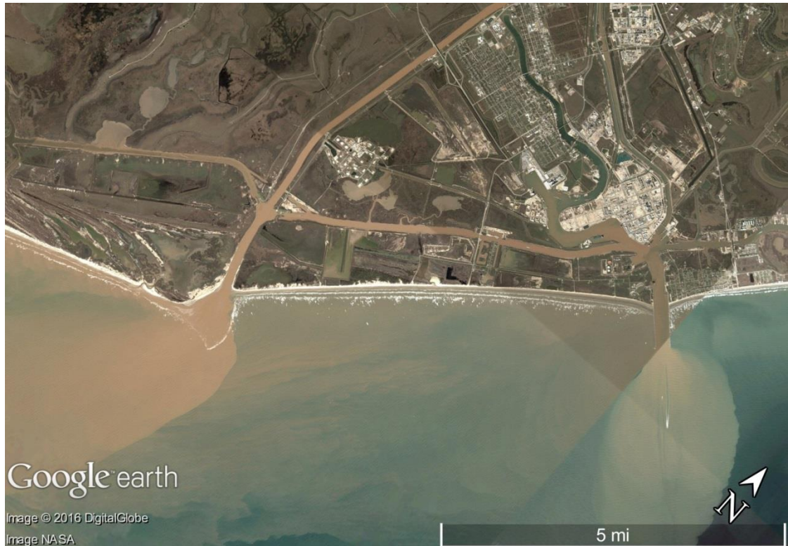
Figure 5 – Flow of suspended sediment from Brazos River to Freeport Harbor Channel, Dec 2004
