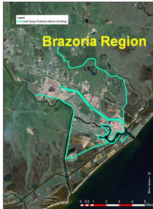
Figure 1: Brazoria Region Hurricane Flood Protection.
