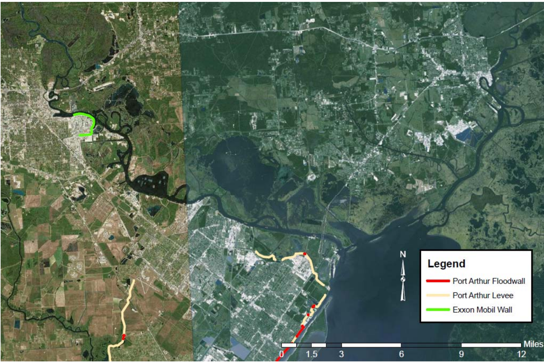
Figure 7-3. Existing Floodwall in the Orange-Jefferson CSRM Project Areas
