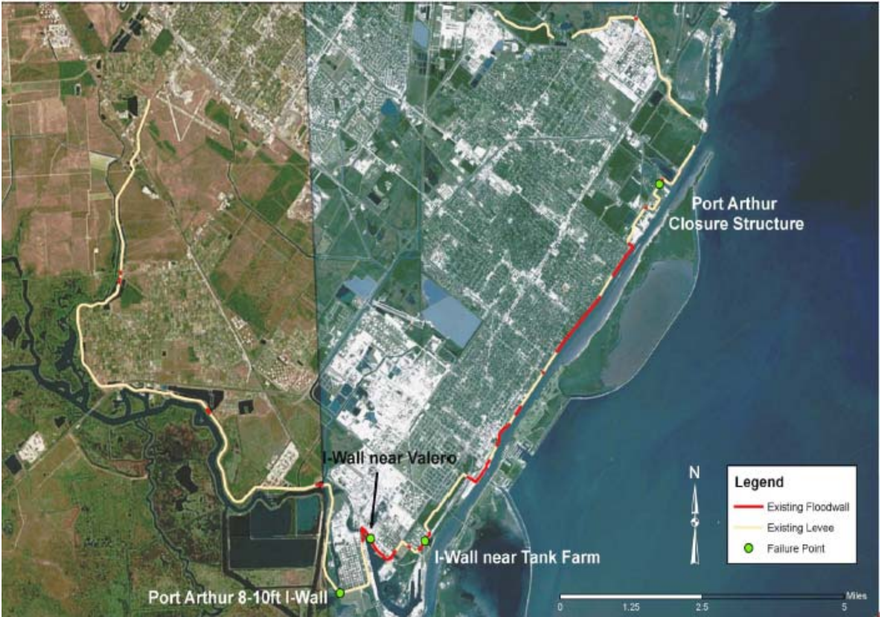
Figure 7-4. Port Arthur and Vicinity CSRM Failure Locations
