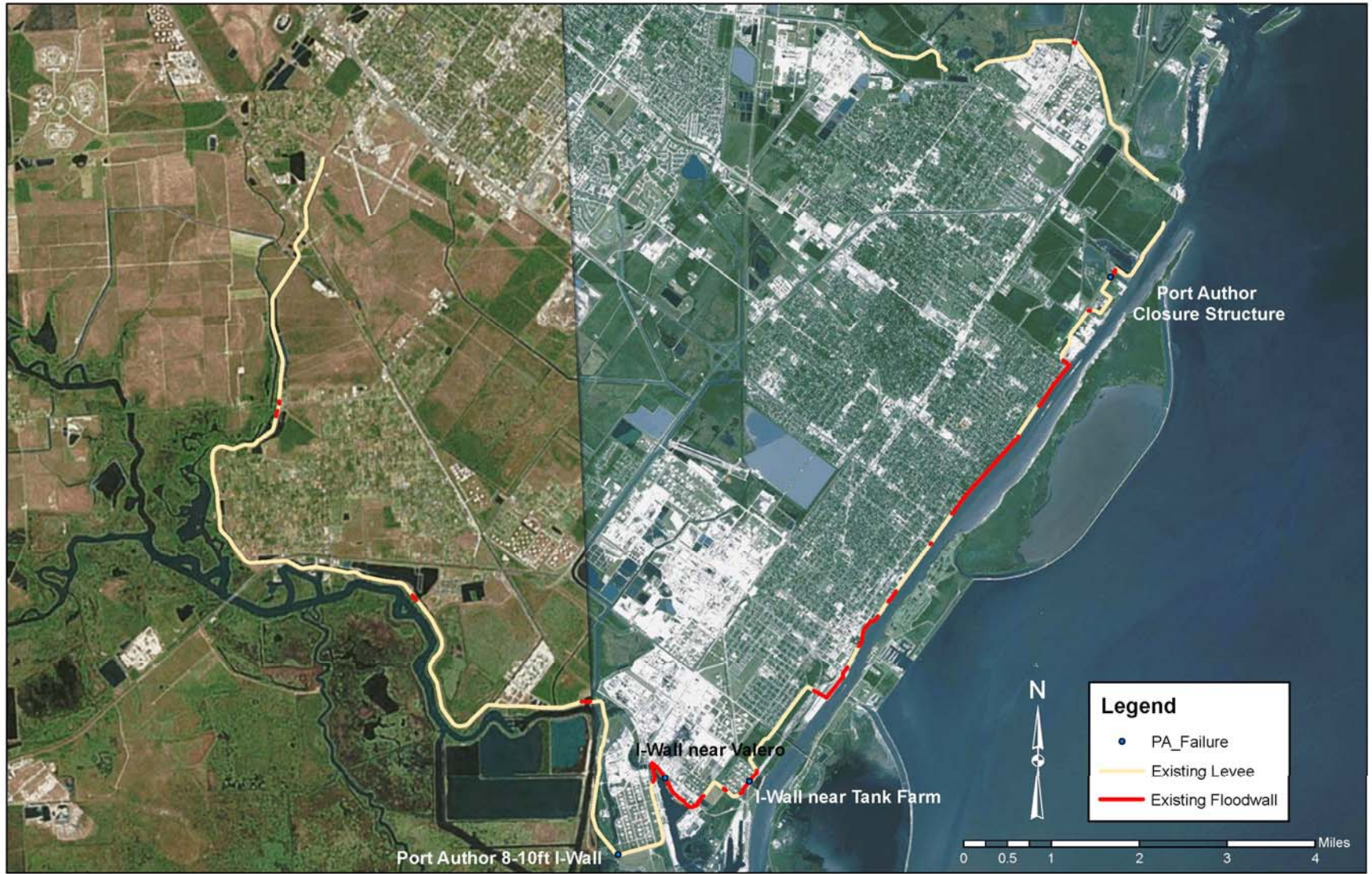
Figure 7-7. Port Arthur and Vicinity Failure Locations
