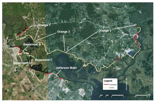
Figure 3-6: Orange-Jefferson CSRM Alternative Reaches
