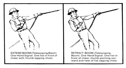
NOTE: Crane signals taken from ANSI/ASME B30 series standards with permission of ASME.
