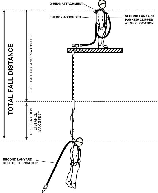
Note: The 12 foot maximum free fall will occur when the tie-off point is at the employee's foot level. If the tie-off point is above the walking/ working level, the free fall distance will be less than 12 feet.
