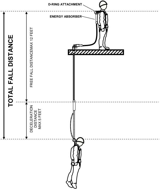
Note: The 12 foot maximum free fall will occur when the tie-off point is at the employee's foot level. If the tie-off point is above the walking/ working level, the free fall distance will be less than 12 feet.
