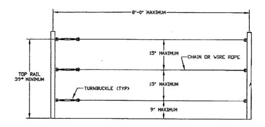
MARINE TYPE B THREE TIER TENSIONED RAILING
