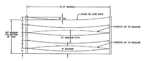
MARINE TYPE C NON-TENSIONED RAILING (3" SAG SHOWN)
