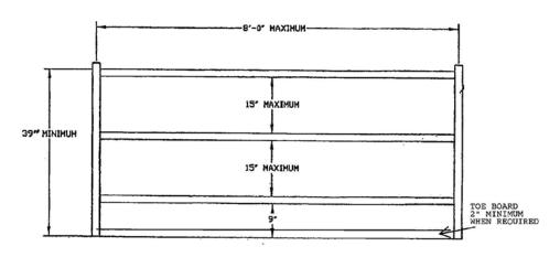
MARINE TYPE B THREE TIER RIGID RAILING
