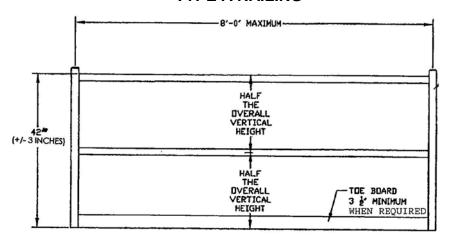
MARINE RAILING TYPE A, TWO TIER RIGID FALL PROTECTION RAILING
