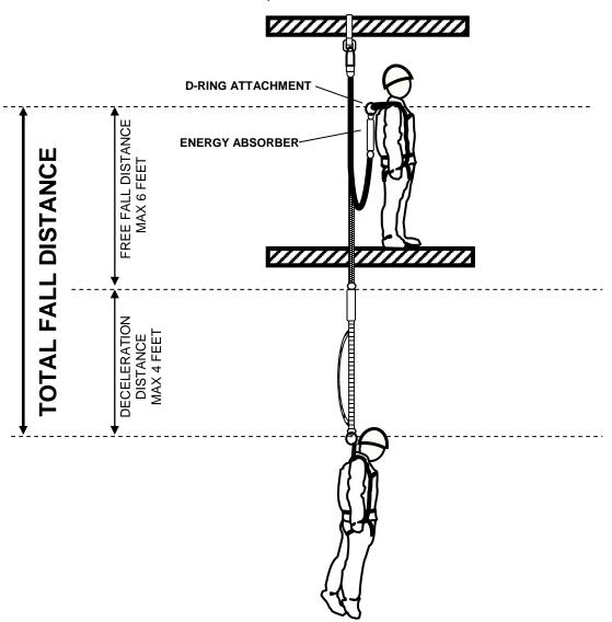
Note: The 6 foot maximum free fall will occur when the tie-off point is at the dorsal D-ring level. If the tie-off point is above the dorsal D-ring level, the free fall distance will be less than 6 feet.
