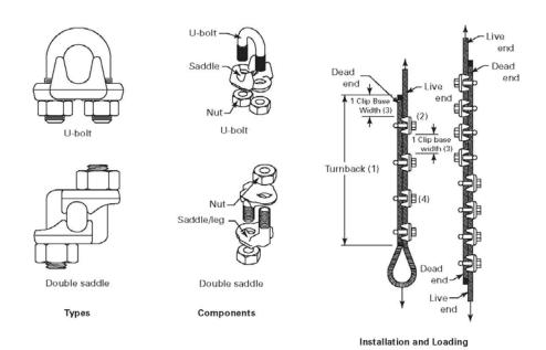
GENERAL NOTE: Correct number of clips for wire rope size shall be used.
