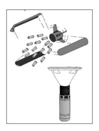
When the fuze in the dispenser functions above the target area, a length of explosive det-cord opens the dispenser container. When that occurs the individual submunitions within the container is spread-out over a large area.
