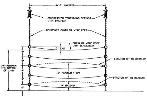
MARINE TYPE C FLEXIBLE/ SWING-AWAY RAILING WITH FLEXIBLE TIERS (3" SAG SHOWN)
