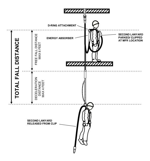
Note: The 6 foot maximum free fall will occur when the tie-off point is at the dorsal D-ring level. If the tie-off point is above the dorsal D-ring level, the free fall distance will be less than 6 feet.
