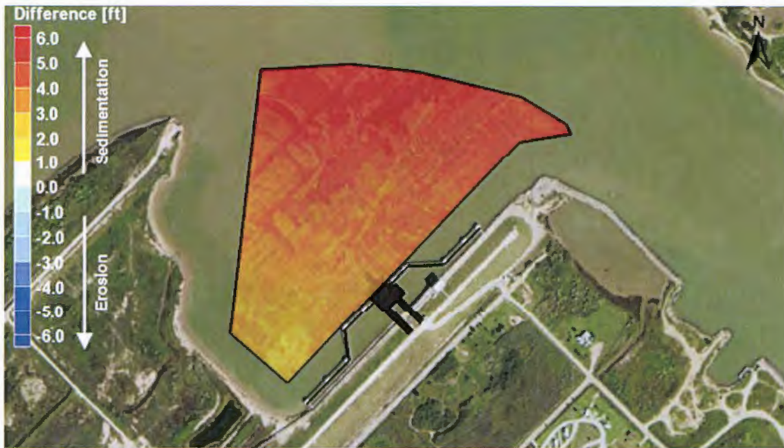
Figure 2 - contour difference plot of the LNG basin between November 28, 2011 and June 7, 2012
