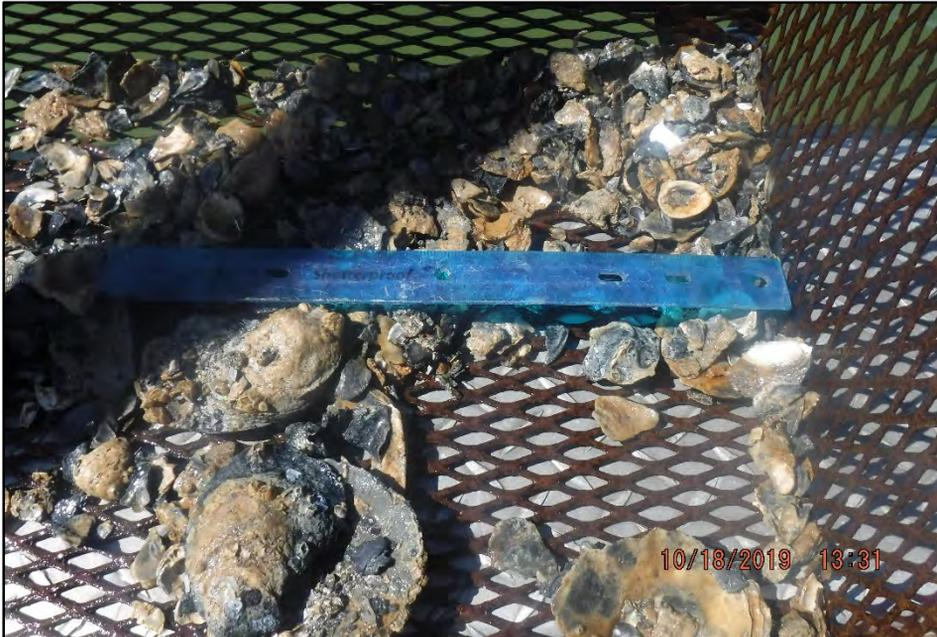
**Photo 30:** Diver Quadrat #05 – post-rinse illustrating the shell hash bottom type that was consistent throughout the project corridor.
