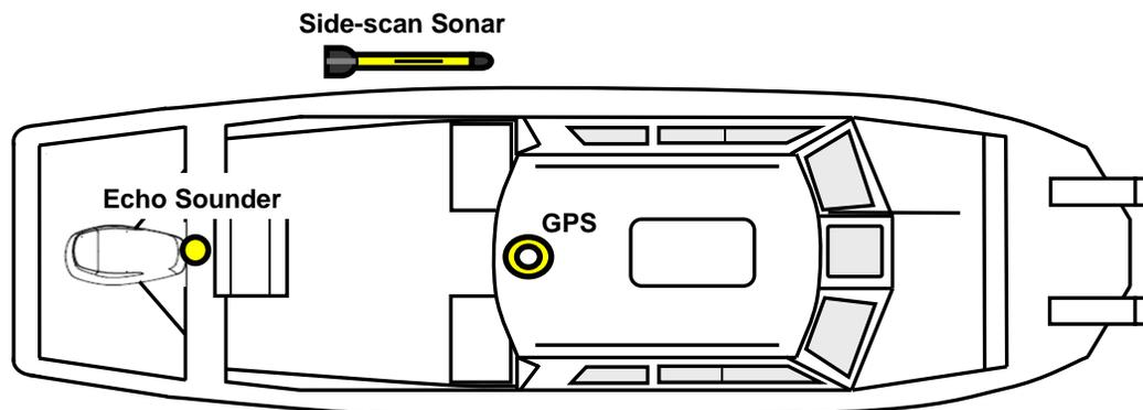
**Figure 1. Equipment layout for the survey vessel.**
