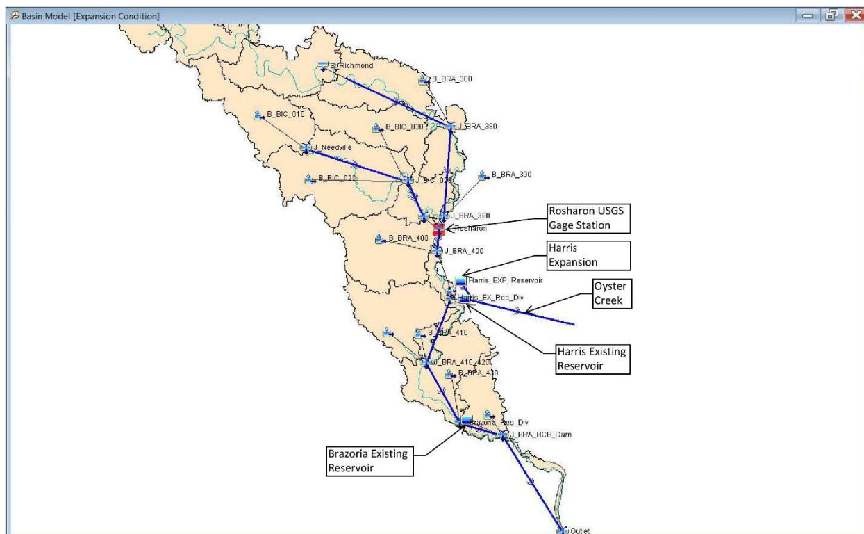
Figure 24: HEC-HMS Model for Harris Reservoir Expansion Project
