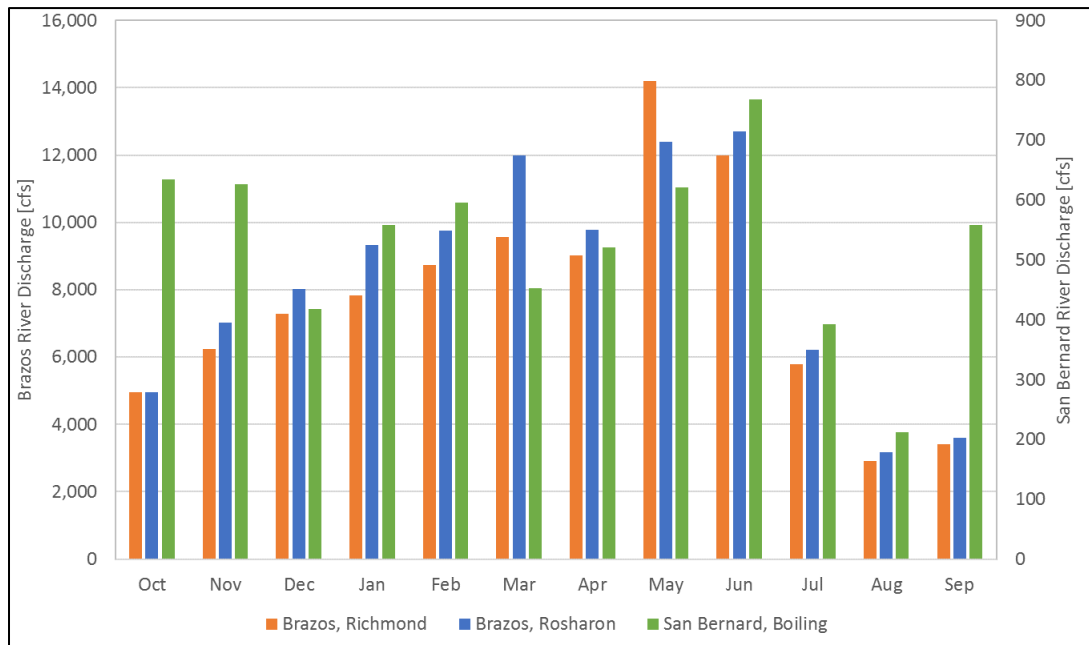
Figure 15: Long-Term monthly mean streamflow discharge at USGS Stations Brazos River near Richmond (upstream in blue), Brazos River near Rosharon (downstream in red) and San Bernard River near Boling. Data are shown in water year from October 1 to September 30.
