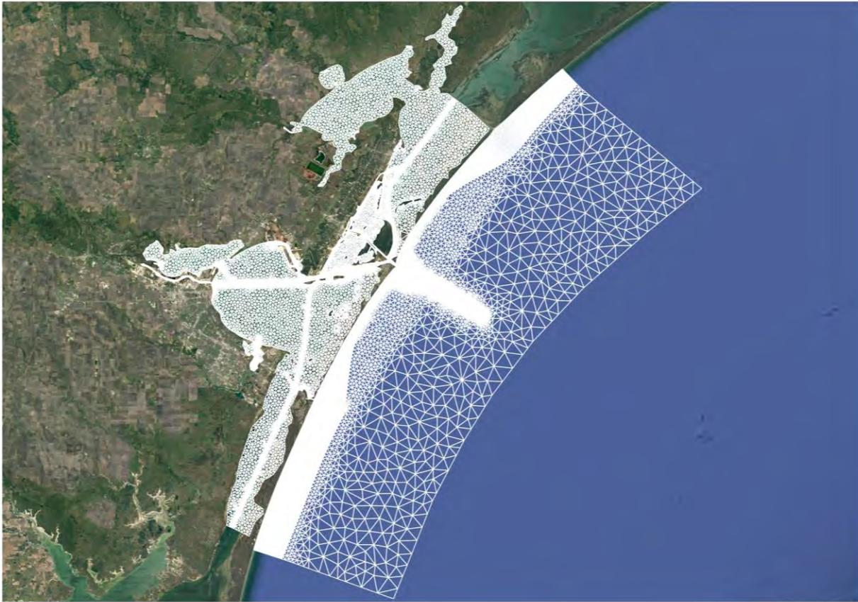
Figure 3.1: Computational mesh for the MIKE sedimentation model
