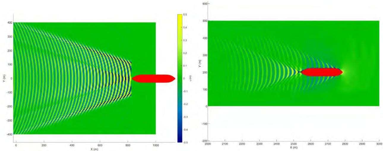
**Figure 4.2: Visual Comparison of the Secondary Wave generated from a VLCC vessel at a speed of 12 knots over an idealized flatbed using the MICHLET solver (left) and FUNWAVE model (right)**
