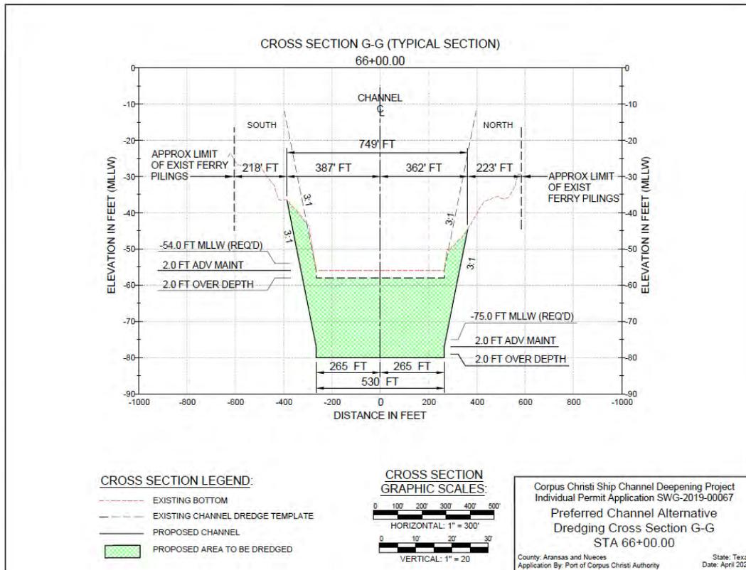
Figure 3.1: Design Section for the Corpus Christi Channel Deepening Project in the Corps Christi Channel (see Figure 1.1 for section location)
