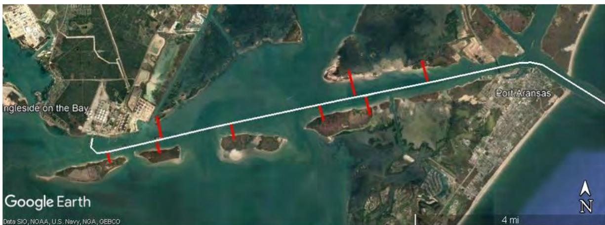
**Figure 2.3: Location of the XBEACH profile models (red) along the Port of Corpus Christi Channel**
