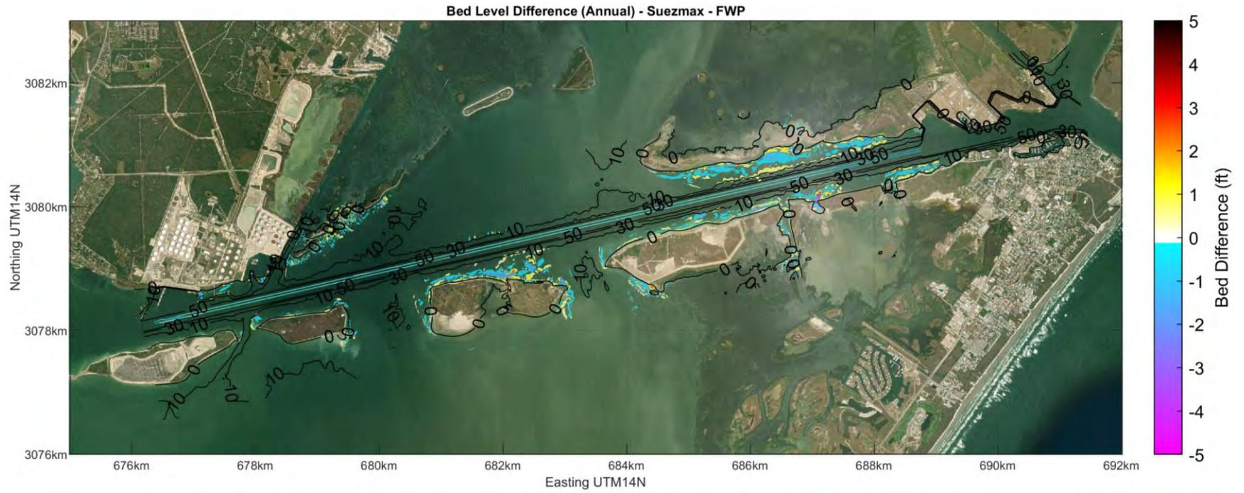
**Figure 5.2: Annualized Bed Level Change under Future With Project Channel Conditions for Suezmax vessel traffic**
