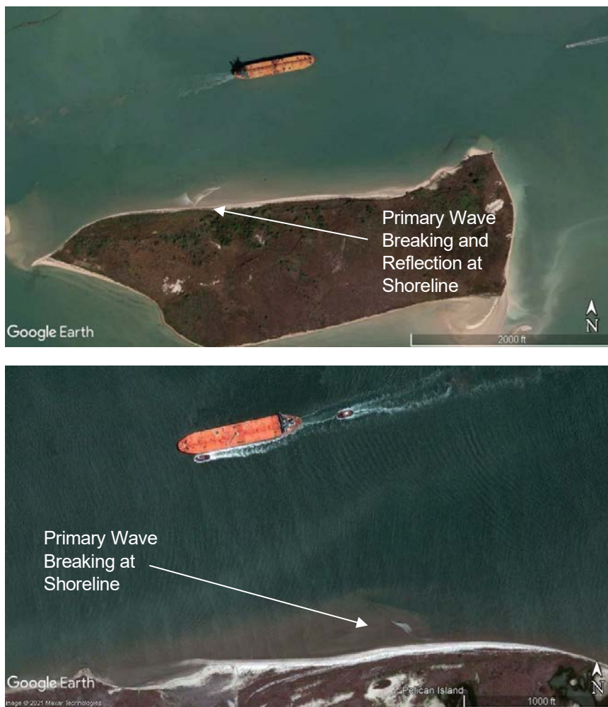
Figure 1.3: Examples of Tanker Generated Primary Waves Breaking along the Shoreline of Corpus Christi Channel
