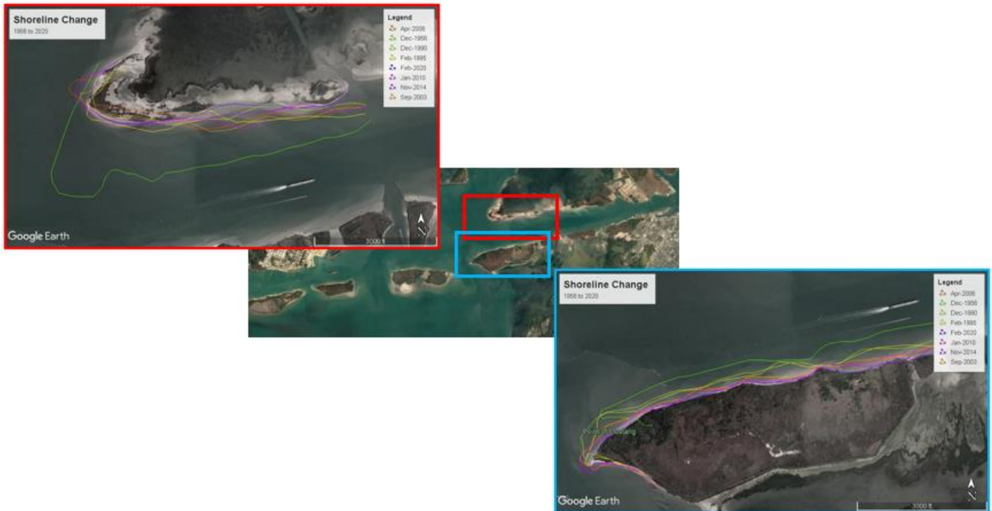
Figure 6.1: Shoreline Position Mapping along a Section of the Corpus Christi Shipping Channel covering the period 1956 to 2020
