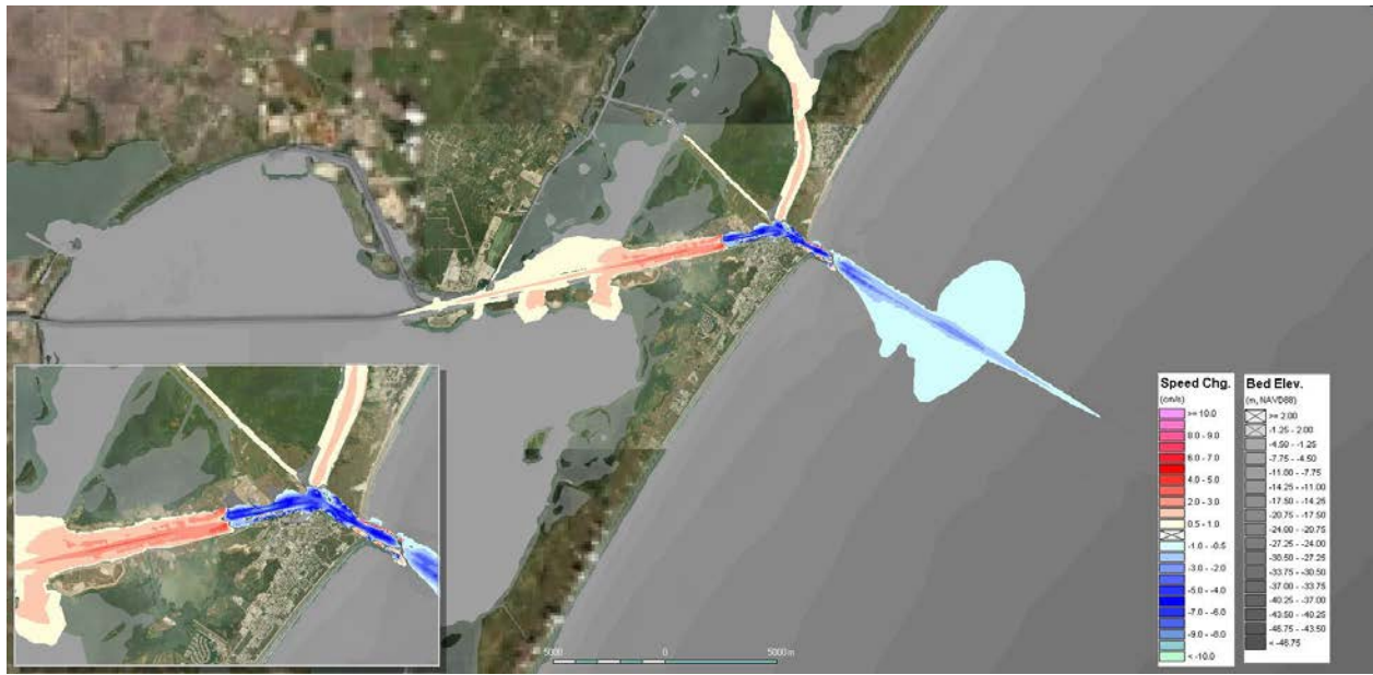
Figure B.24: Depth averaged speed change caused by the FWP in Period 1
