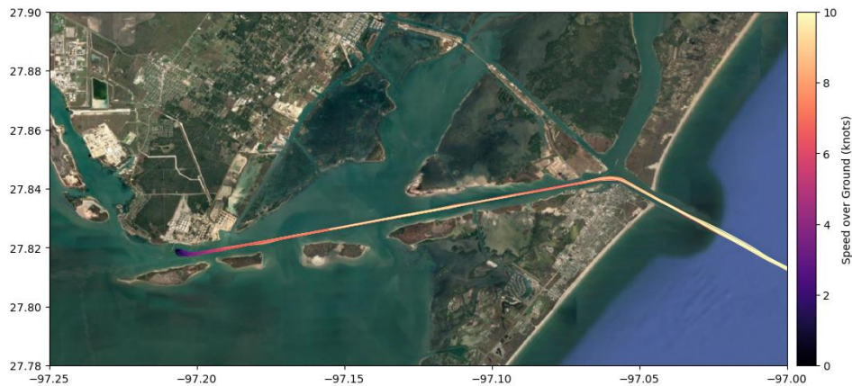
Figure 3.4: Tracks and speed profiles of outbound transits from the Ingleside terminal from AIS data for VLCCs and Suezmaxs (2019 – 2020)
