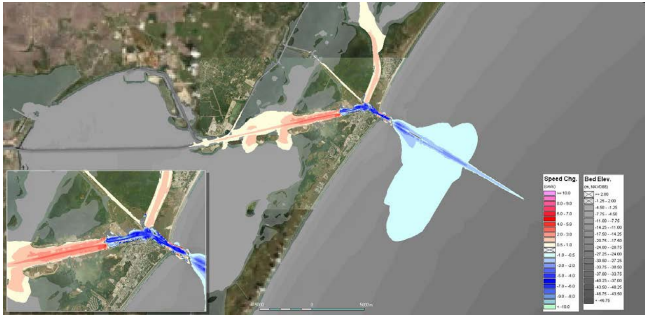
Figure B.26: Depth averaged speed change caused by the FWP in Period 3
