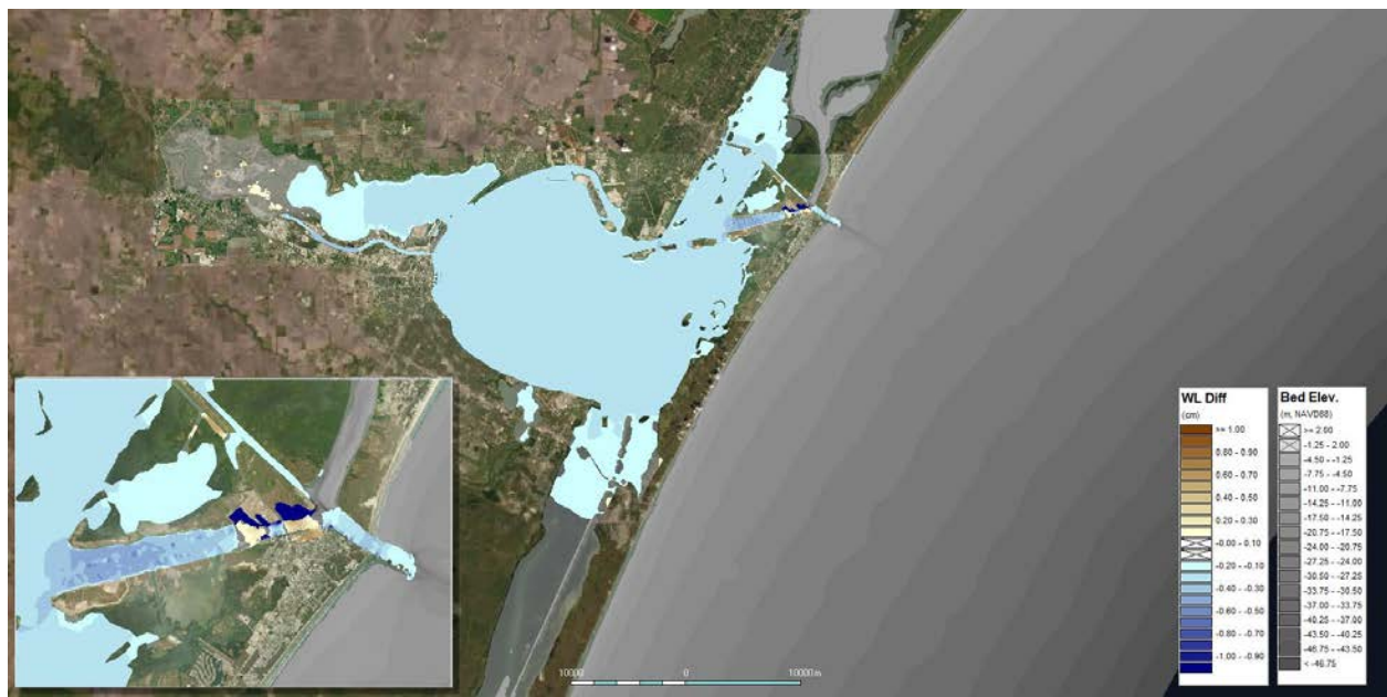
Figure 5.1: Impact of FWOP on mean water levels compared with existing conditions
