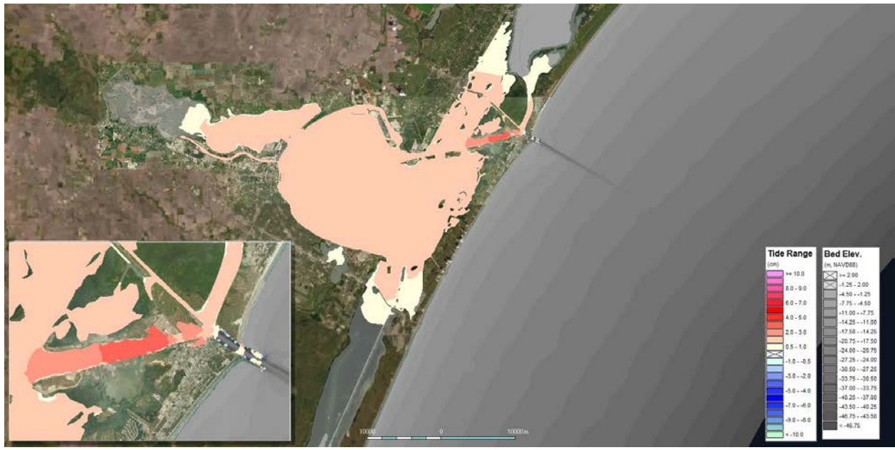
Figure 4.20: Mean tide range change caused by the FWP relating to the FWOP
