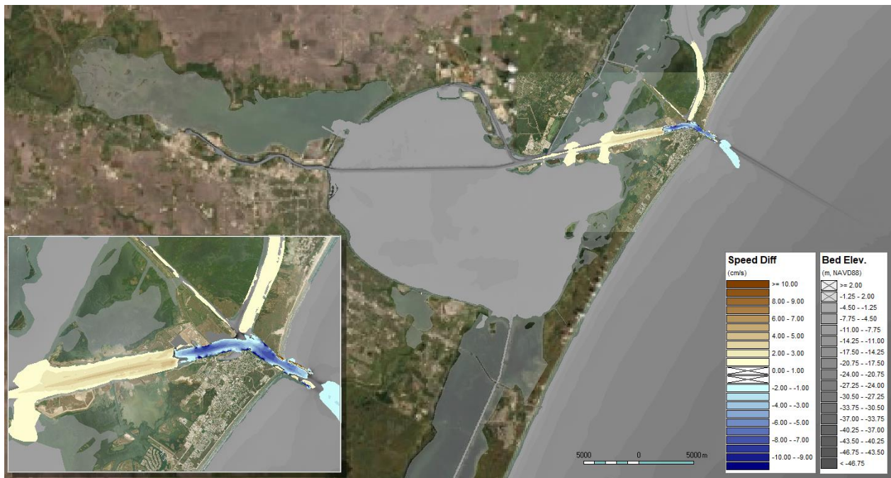
Figure B.33: Average flow speed change on water surface in Period 3
