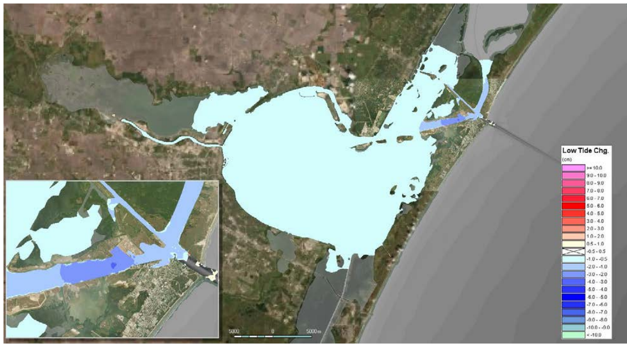
Figure B.7: Average change of low tide caused by the FWP in Period 1
