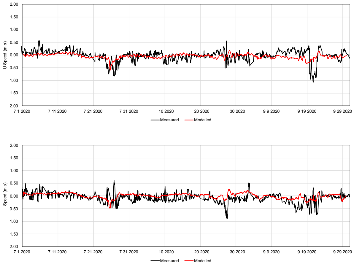
Figure A.26: Comparison of model predicted flow velocity components, U (east) and V (north), with the measured data at TABS-D during Period 3
