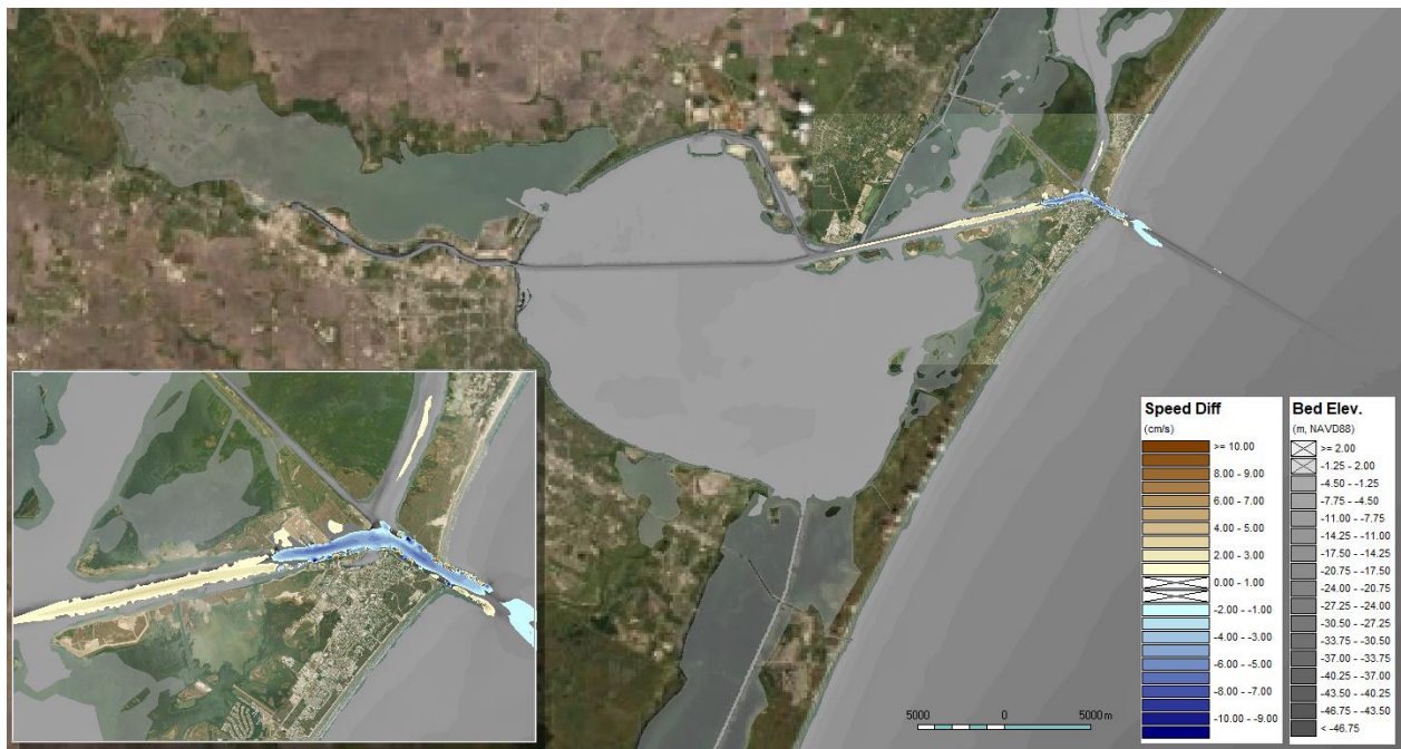
Figure B.29: Average flow speed change at the elevation of -10 m (NAVD88) in Period 1
