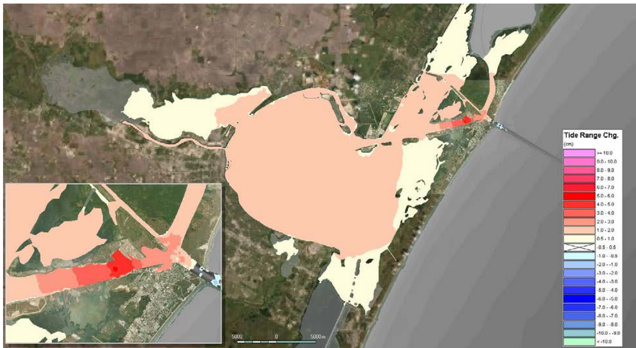
Figure B.19: Average Change of Tide Range Caused by FWP in Period 2
