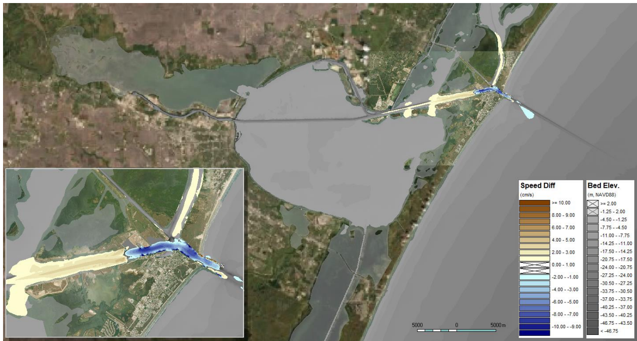
Figure B.27: Average flow speed change on water surface in Period 1
