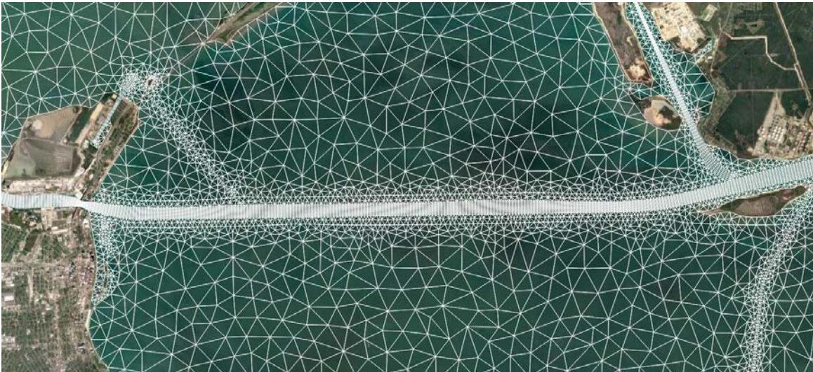
Figure 3.2: Computational mesh for the MIKE sedimentation model showing the grid cells in the channel
