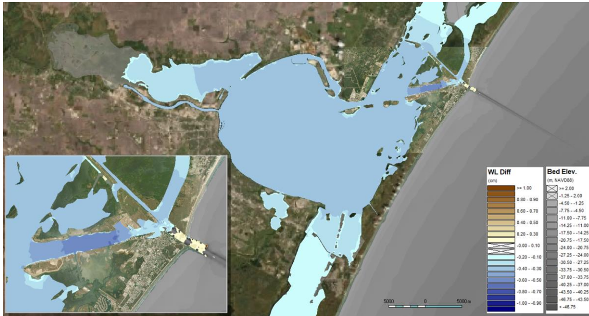
Figure 4.5: Impact of FWP to mean water levels as compared to FWOP during Period 2
