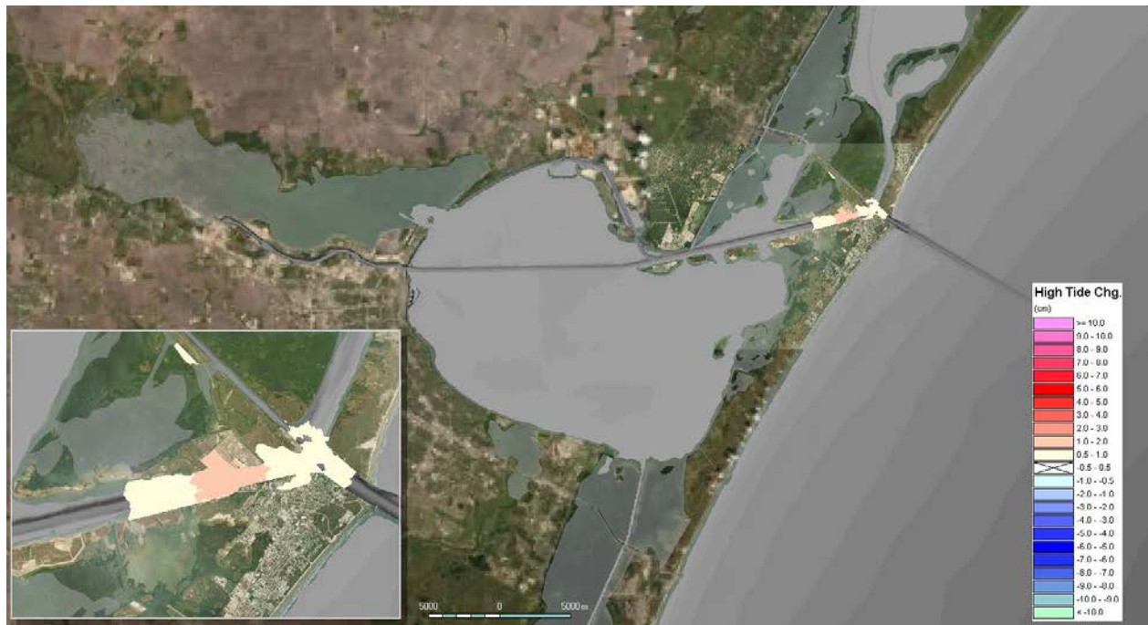
Figure B.5: Average change of high tide caused by the FWP in Period 2
