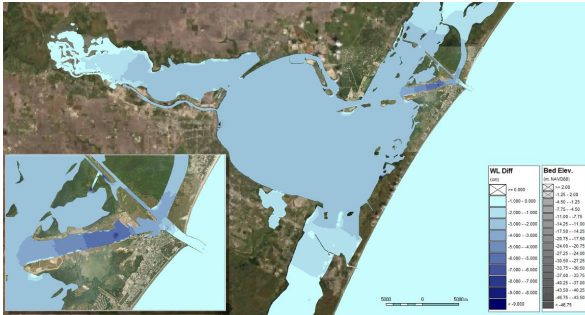
Figure 4.8: The average drop in low tide caused by the FWP in comparing with the FWOP in Period 2
