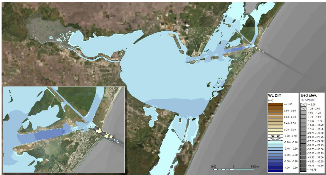
Figure B.3: Change of mean water level caused by the FWP in Period 3
