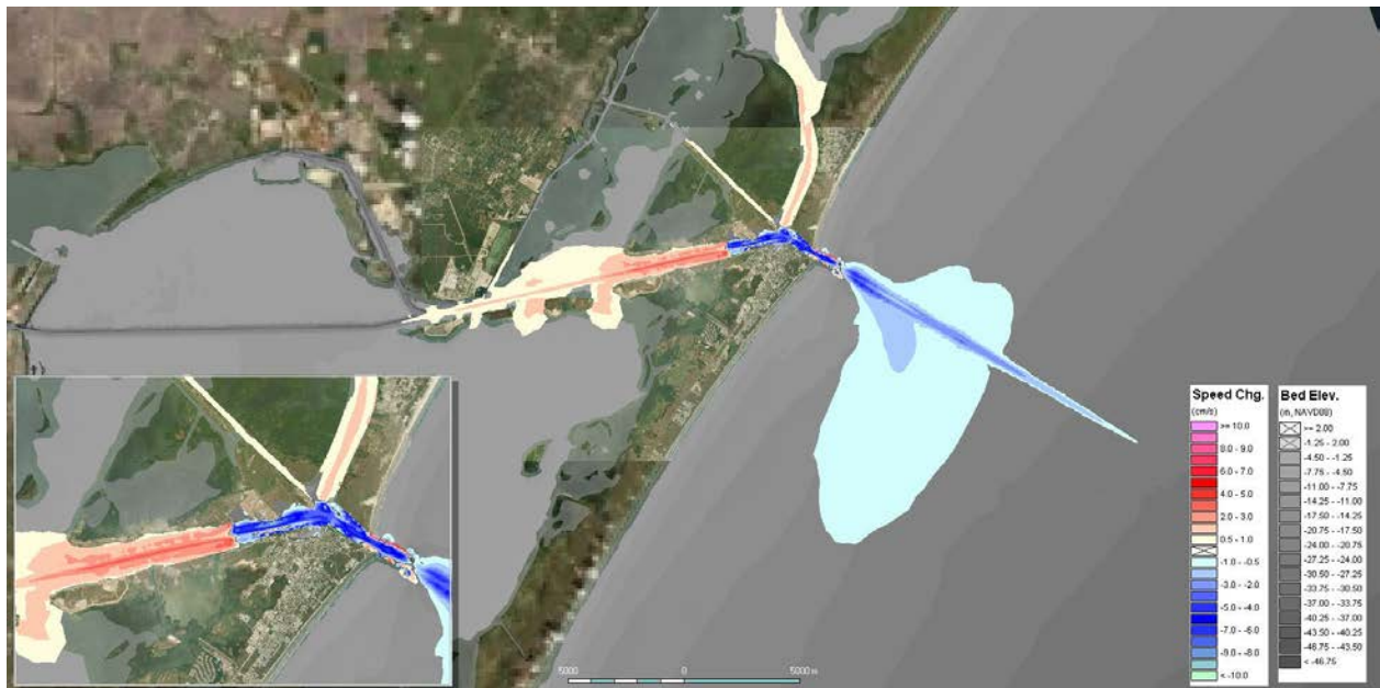
Figure B.25: Depth averaged speed change caused by the FWP in Period 2
