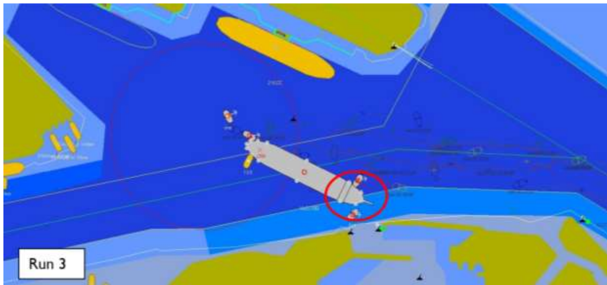
Shows stern of VLCC aground with medium flood velocity at the intersection
