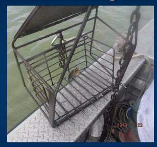
Frame: constructed with 13 mm diameter cold rolled steel rod 495 mm wide × 241 mm high × 1,000 mm long.
